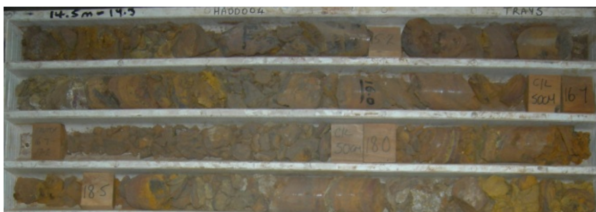
Plate 14: core photograph of a section of Goethite-hematite-rich zone in the Marra Mamba Formation (16.7 – 17.2 m) in hole HADD004. A cavity was noted from 16.7 to 17.2 m.
