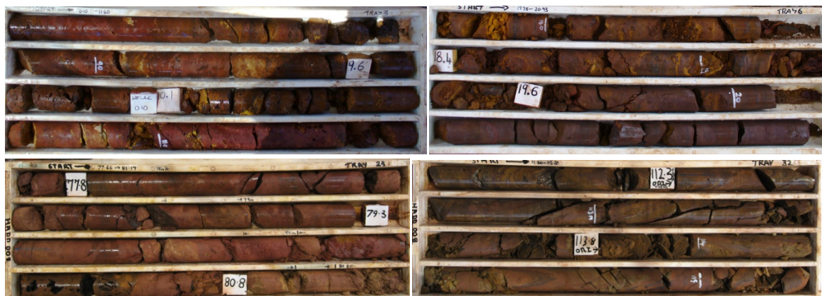
Plates 20 – 23: Prospective troglofauna habitat in the pisolitic duricrust (8.1 – 11.6 m) and Goethite (17.75 – 20.93 m) and in Goethite-hematite sections (77.66 – 81.77 m) and BIF (111.8 – 1151.28m) from HADD008, located in the Brockman Formation.
