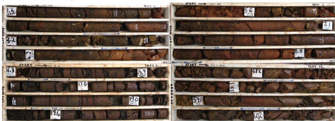
Plates 24 – 27: Prospective troglofauna habitat from HADD009. Plates 17 and 18 show sections with large vugs within the upper levels of the profile (mottled duricrust, 1.4 – 5.1 m and 5.1 – 8.91 m) while Plates 19 and 20 show prospective habitat in the goethite-hematite sections (16.3 – 20.02 m) and silica-rich BIF.
