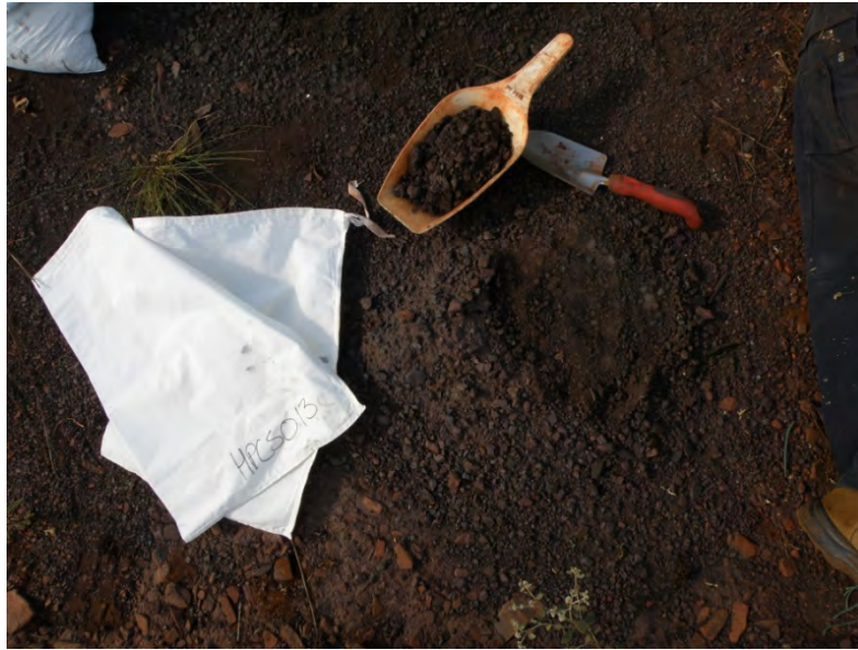
Figure 4 : Outer skin of sample pile is collected as it is removed from this high sulphur Whaleback Shale sample.
