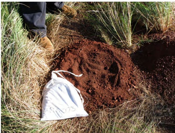
Figure 3 : A sequence of photos demonstrating the sampling technique. The outer skin of the pile is moved to the side (top) exposing the inner core (middle) and the sample is then taken (bottom).
