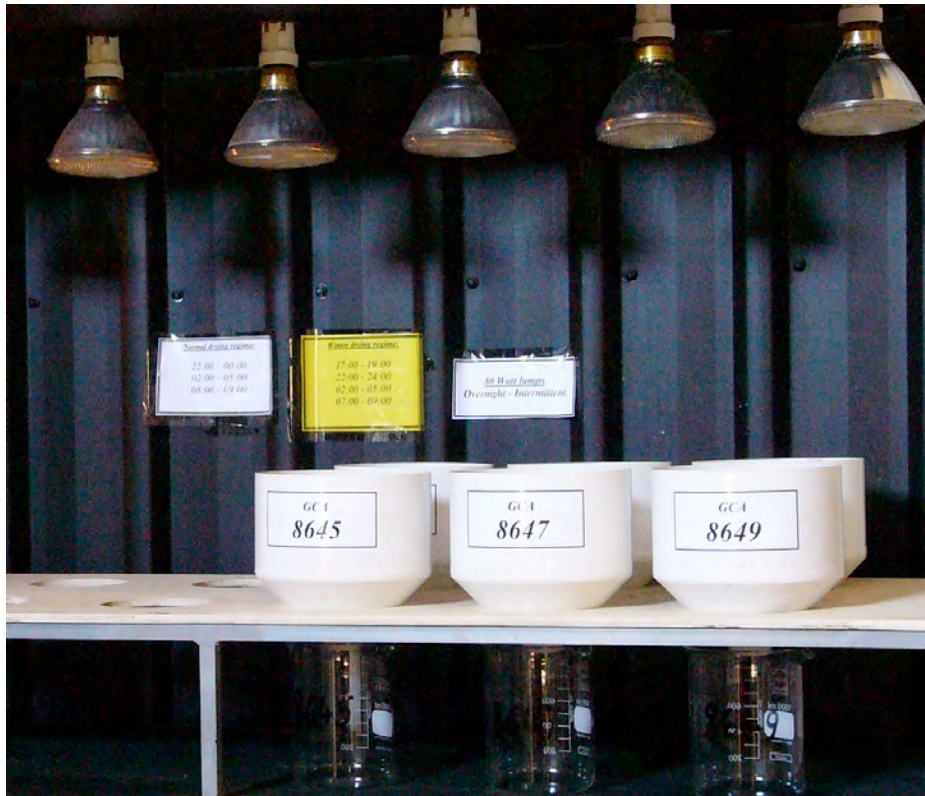
Plate 1a: Typical Weathering-Column Assembly
