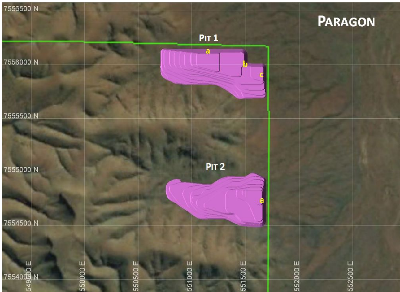
Figure 8: Paragon Pits, highlighting areas of geotechnical risk (refer to Table 12 and Table 13)
