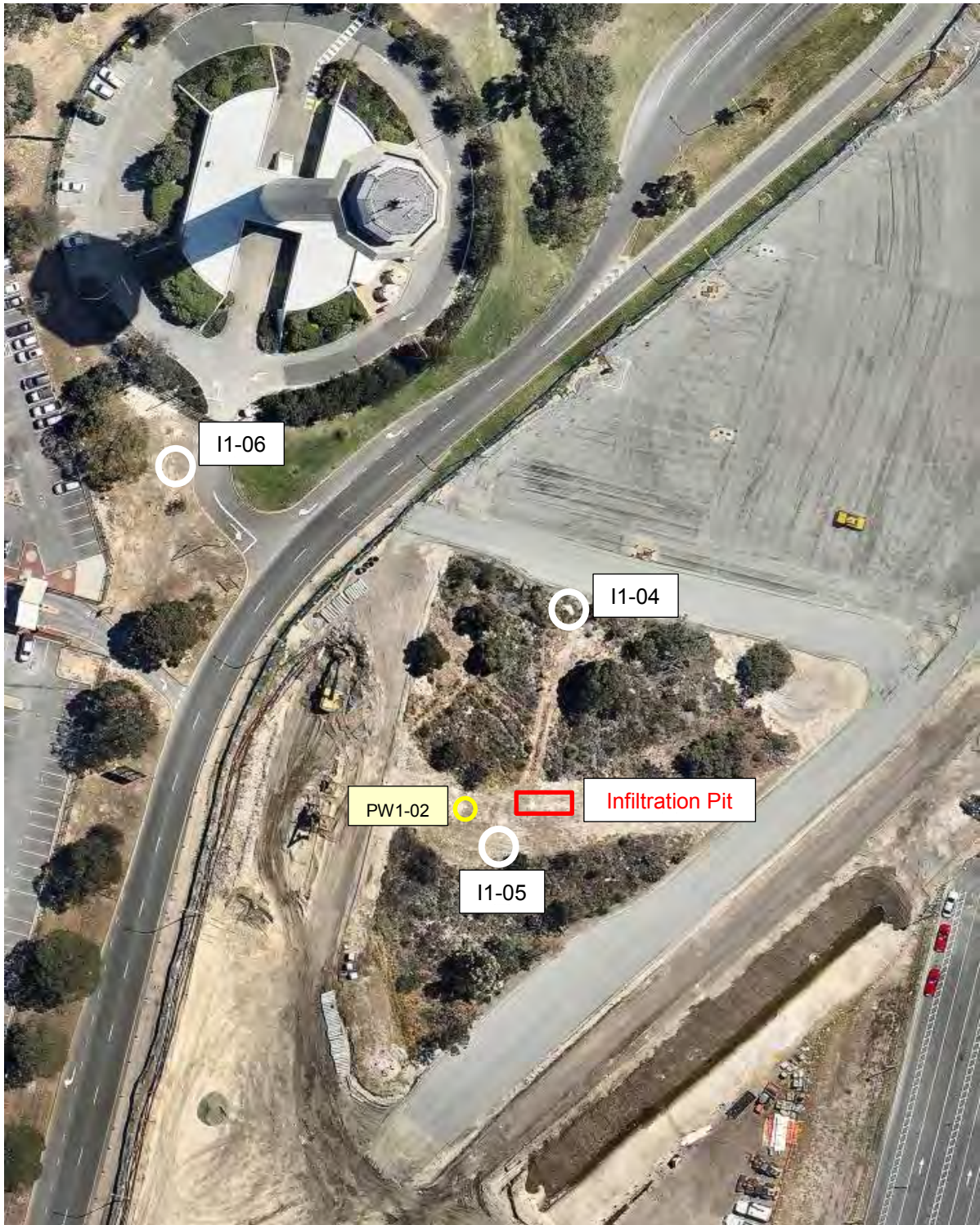
Infiltration Test Locations at Consolidated Airport Terminal Station
