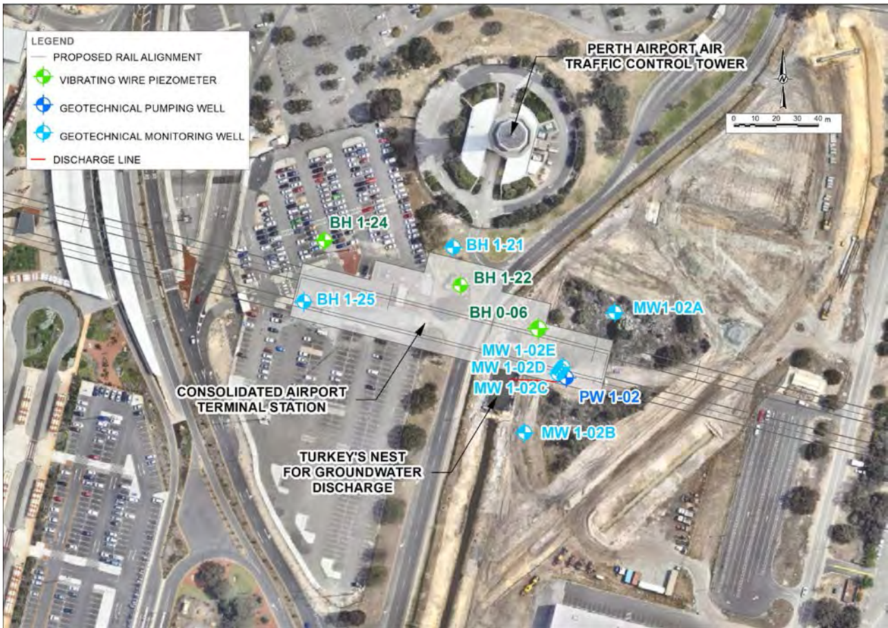
Sketch 2: Site Layout for pumping test at PW 1-02
