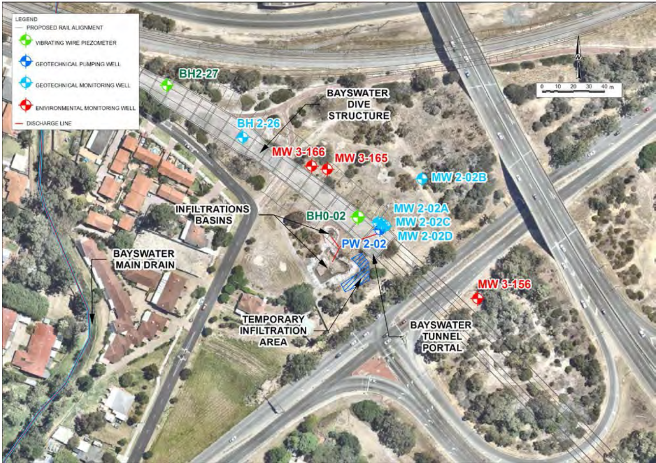
Sketch 4: Site Layout for pumping test at PW 2-02
