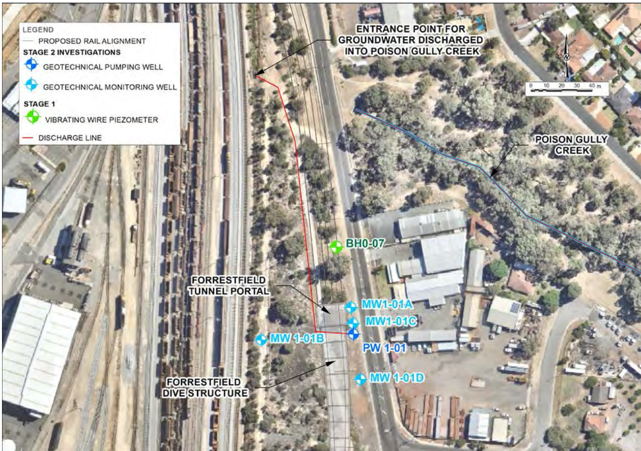
Sketch 1: Site Layout for pumping test at (PW 1-01)
