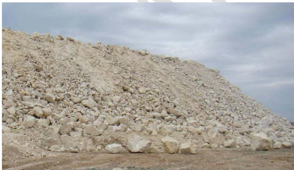
Figure 4-8: Blasted sandstone at Ellendale mine (boulders in foreground ~1m diameter)
