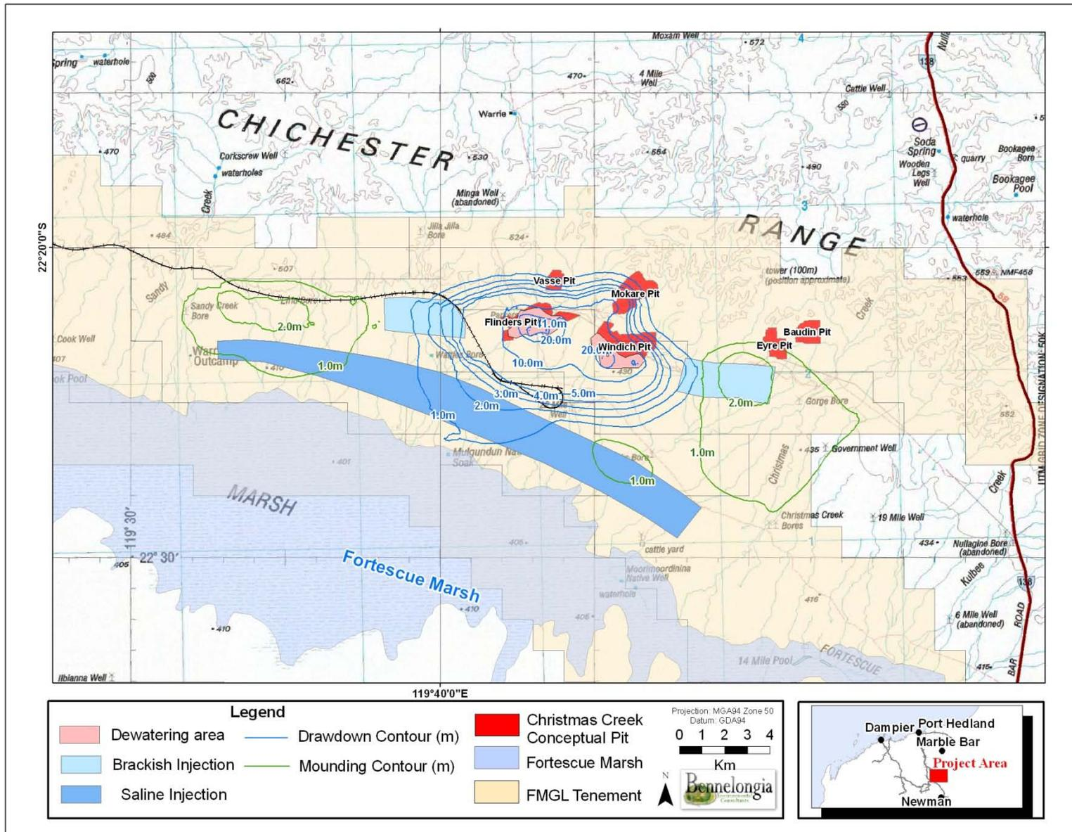
Figure 4. Location of borefields at Christmas Creek and modelled groundwater abstraction/injection (mounding) contours.
