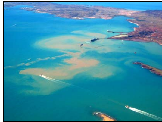
Dredge plume. Parker Point, Dampier, June 2004.
