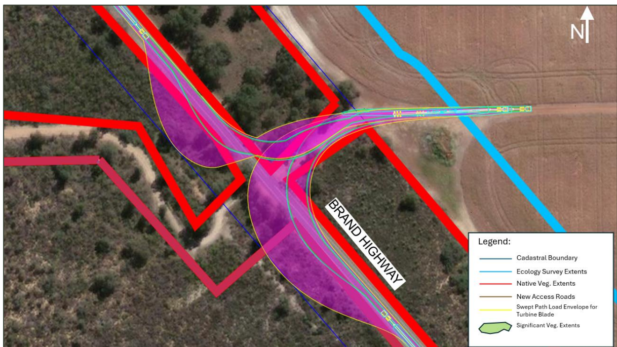
Figure 7-7: Turnaround/ Brand Highway swept path analysis
