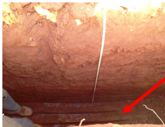
UWA Pit 9 - Soil profile with massive, impenetrable silcrete at depth (inset)
