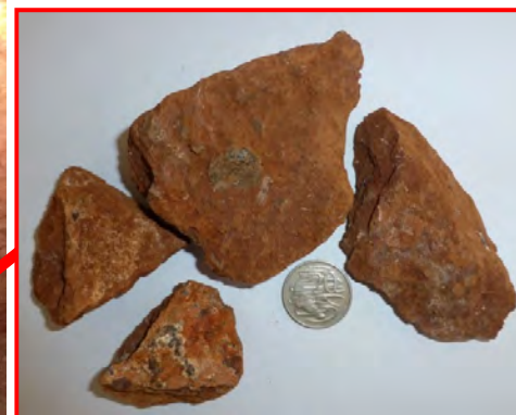
UWA Pit 9 - Soil profile with massive, impenetrable silcrete at depth (inset)
