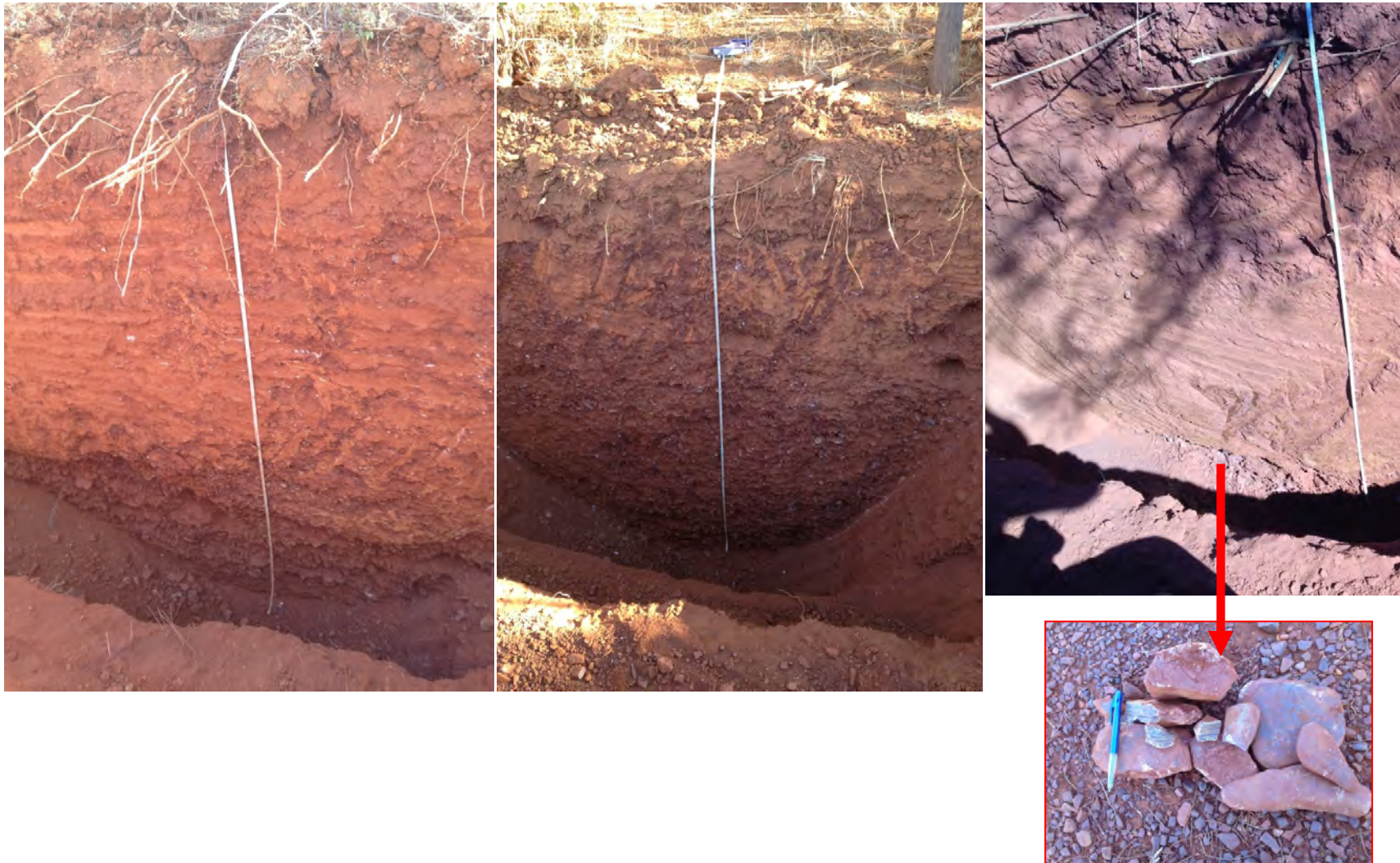
Figure 4 Soil profiles in mulga lined drainage tracts north of the Fortescue Marsh, showing cobble layers at depth
