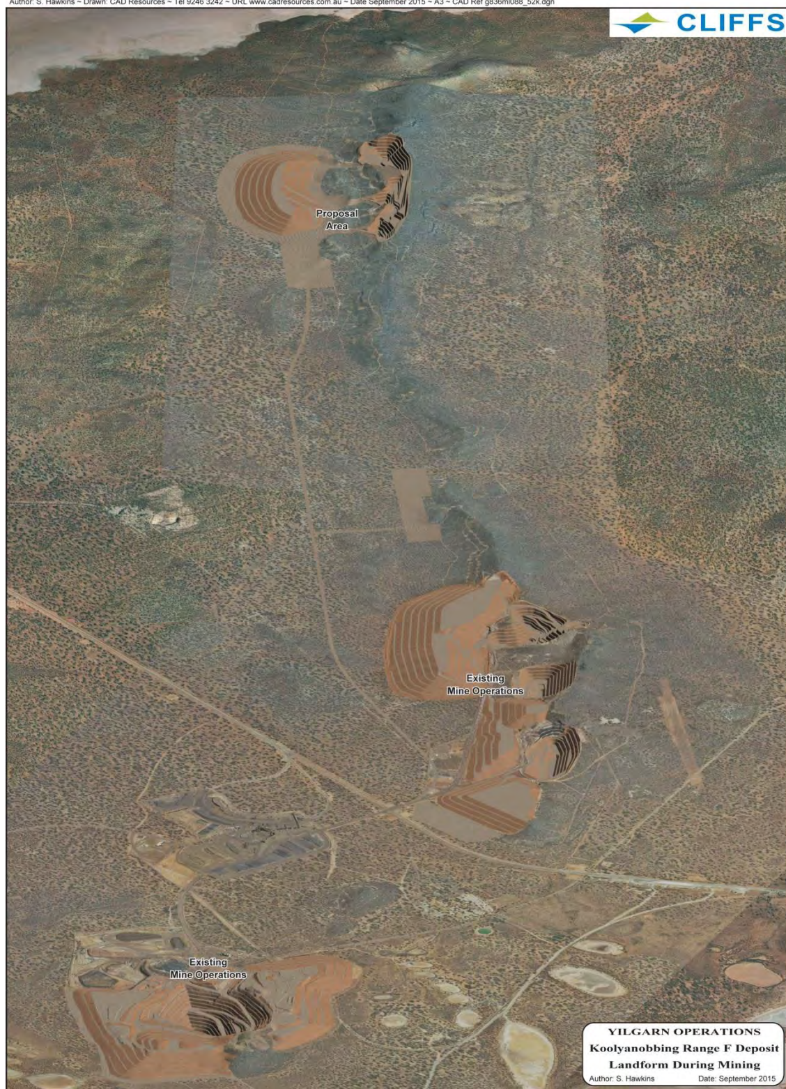
Figure 3-25b Conceptual Landforms during Mining. The conceptual image identifies the landforms of the southern Koolyanobbing Range during mine operations, as viewed from the northern side. The Proposal area is identified in yellow. The Proposal and the approved Koolyanobbing Range mine operations are identified at full development, prior to mine closure.
