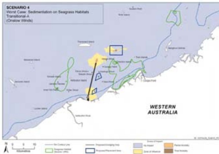
Figure B.188 Scenario 4, Transitional-A, Worst Case: Sedimentation Zones of Impact for Seagrass during Transitional Conditions with Worst Case Spill based on Onslow winds
