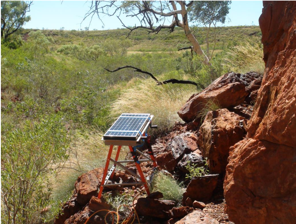
Plate 3: Typical installation of the solar panel providing power to the SM2 detector at Cave 13.
