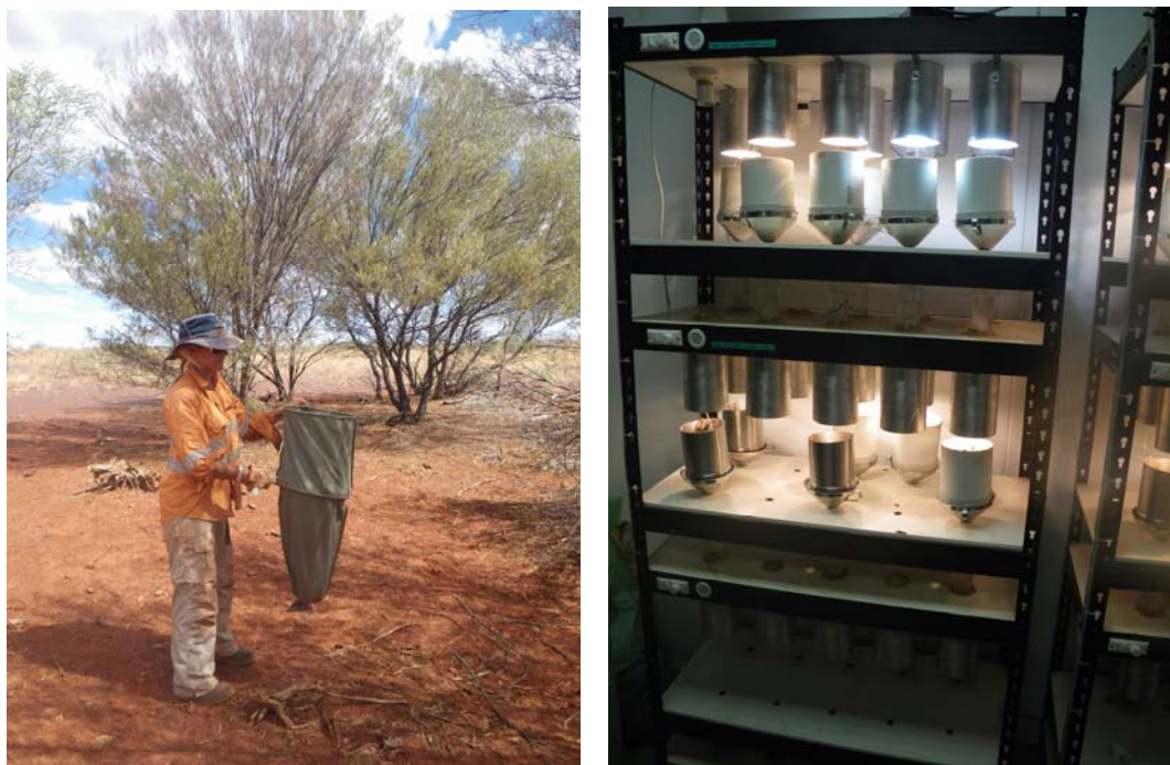
Figure 3.3 – Examples of the Leaf Litter Redcuer and Tullgren Funnels
