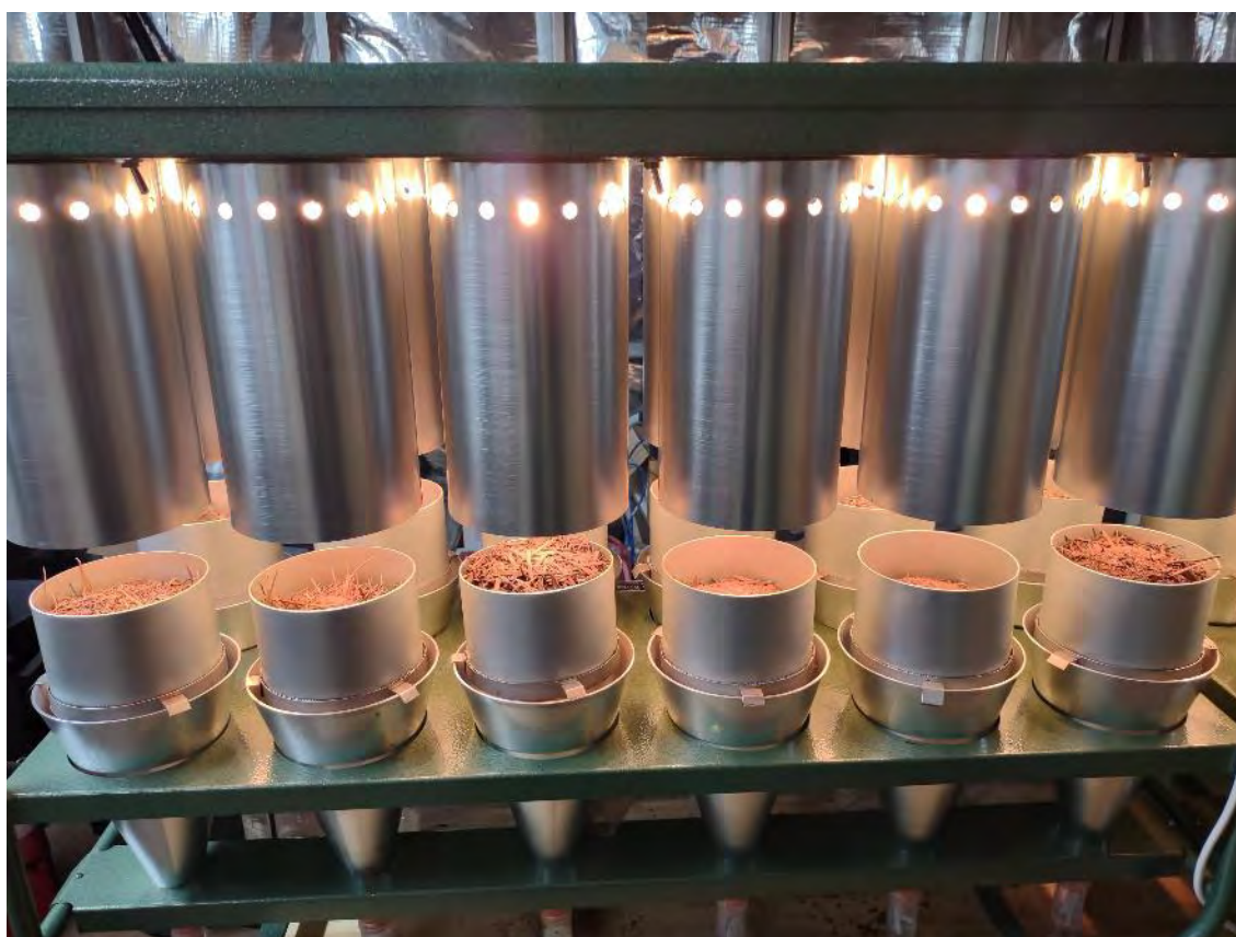
Figure 3.2: Tullgren Funnels for Extraction of Invertebrate Specimens
