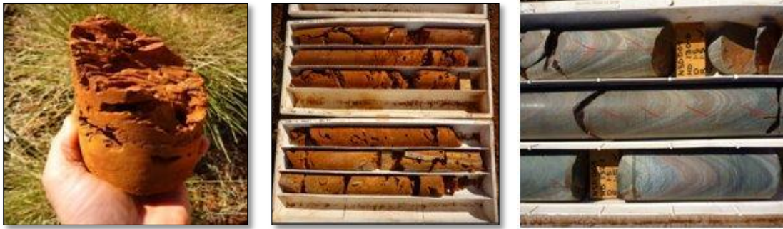
PLATE 7: Prospective troglofauna habitat at North Star showing well developed secondary porosity in shallow subsurface BIF (top right and left) and total absence of porosity / cavities in deeper sections (lower) (Photos Subterranean Ecology taken at the North Star prospect July 2011).
