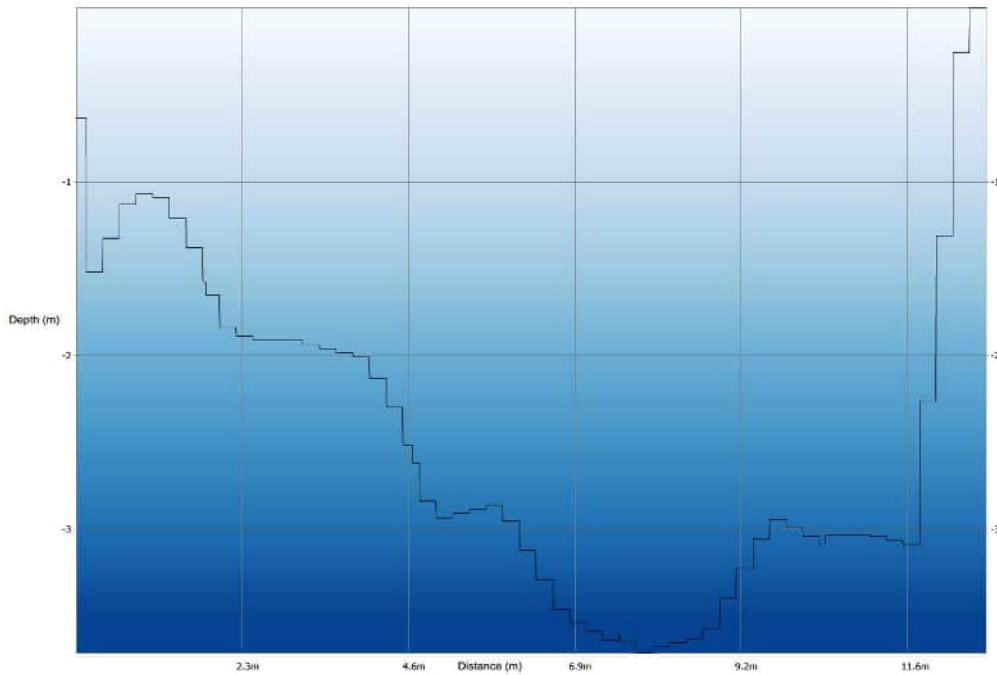
Figure 3-35 Cross-section of deep southern portion of Mundagoora Pool (East-West)
