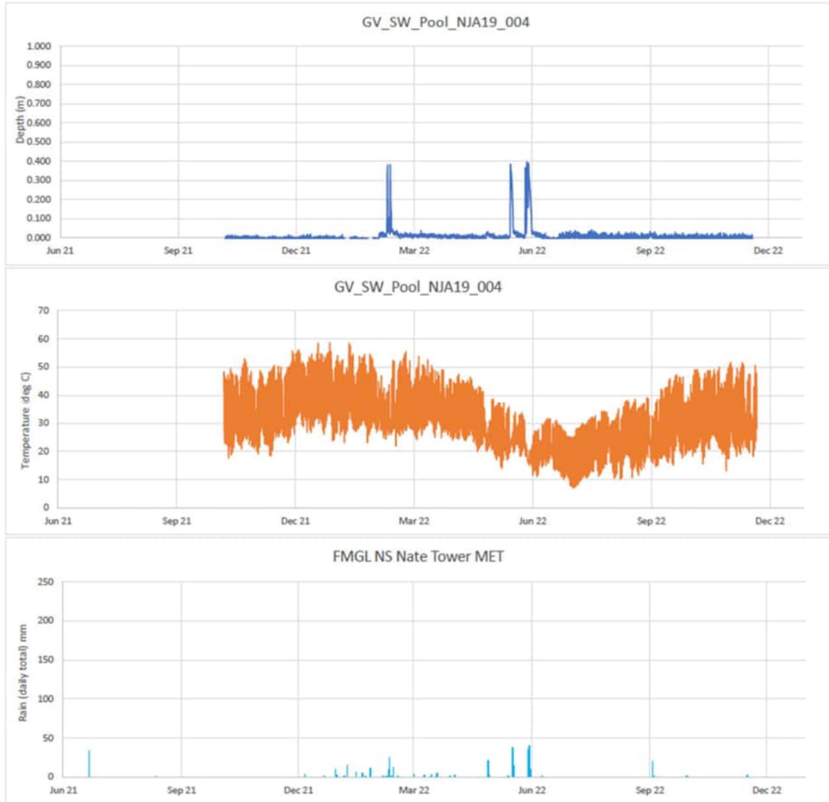
Figure 3-98 NJA19_004 Pool logger record from 7/10/2021 to 07/12/2022 for pool water depth (m), water temperature (°C), and daily rainfall at FMG LNS Nate Tower MET.
