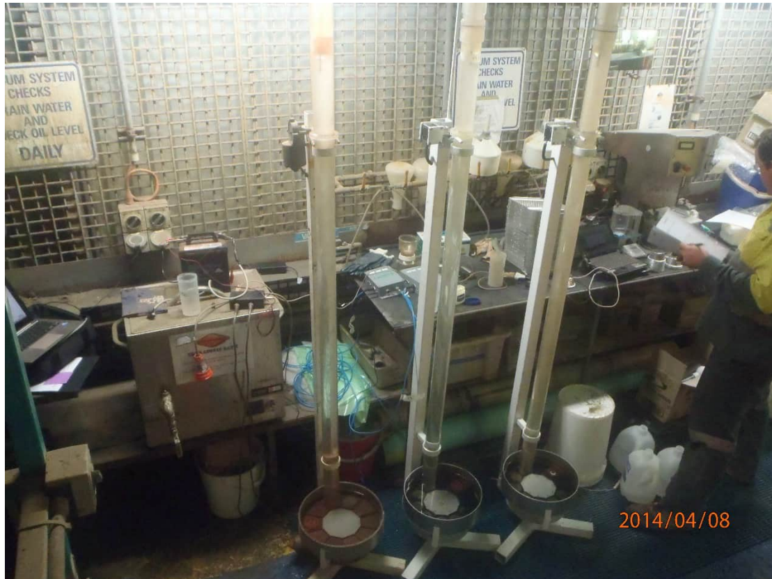
Figure 3: Landloch's automated settling columns deployed on site in support of field-based rainfall simulation.
