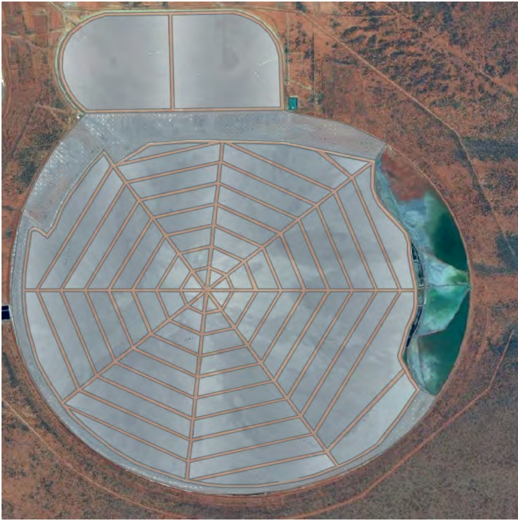
Figure 11: Example of cell bunding on a Convex TSF as proposed for Yangibana
