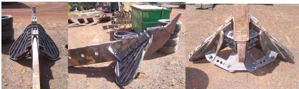
Figure 14: Example of adjustable winged tines to produce deep wide rip lines
