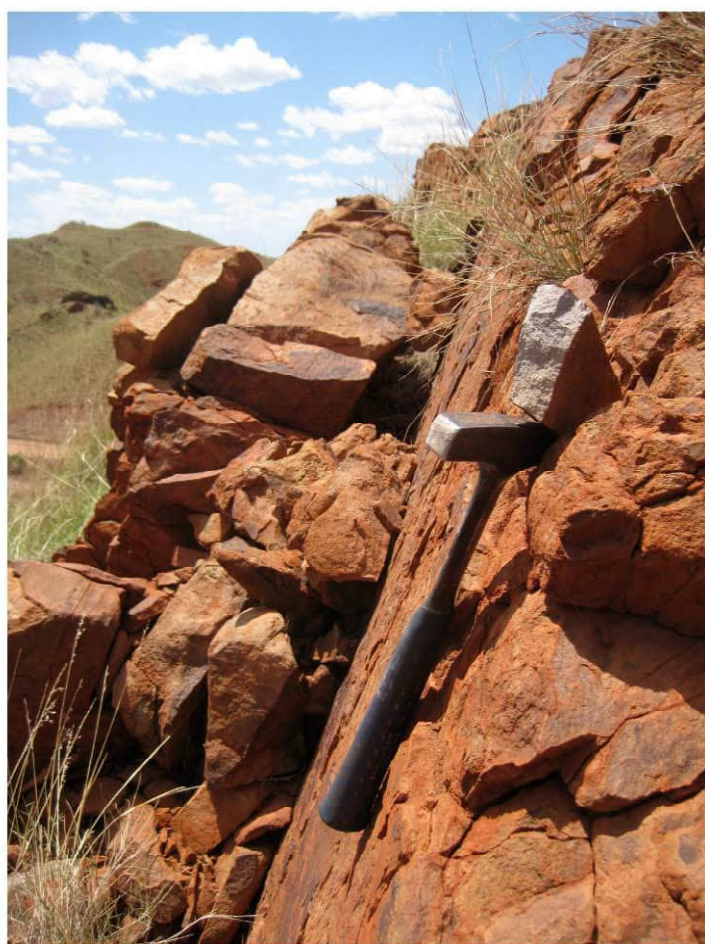
6. 75/245 joint set in sandstone
