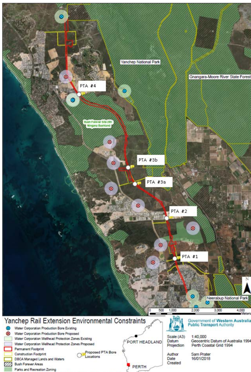
Figure 3 Proposed PTA Construction Groundwater Abstraction Bores
