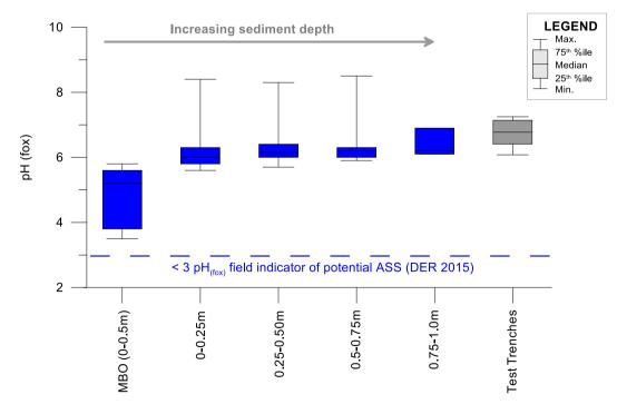
Figure 4 Chemically oxidised pH (pH<sub>fox</sub>) with increasing sediment depth across all sites, including test trench water pH for reference
