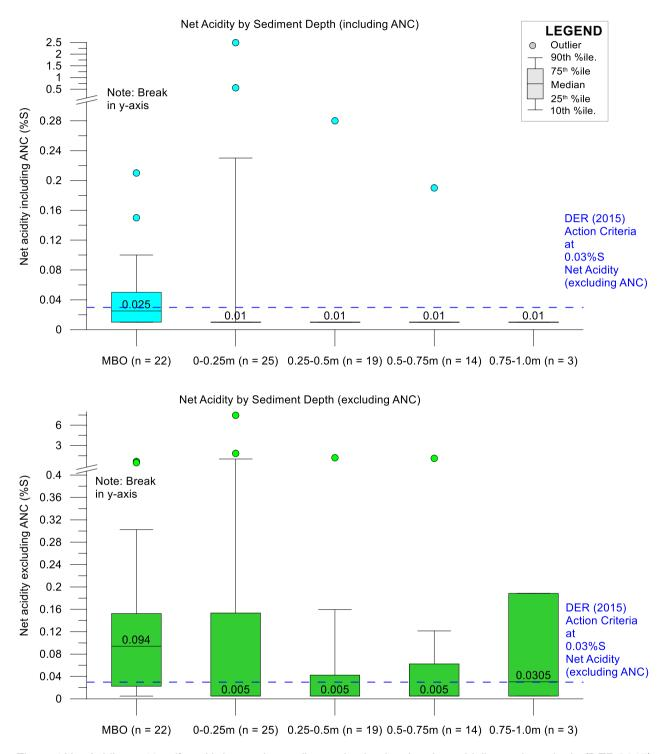
Figure 1 Net Acidity as % sulfur with increasing sediment depth, showing the guideline action criteria (DER 2015); o symbol indicates outliers (factor 1.5) – including (top) and excluding (bottom) acid neutralising capacity (ANC) respectively
