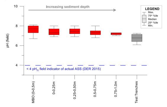
Figure 3 Field pH (pH<sub>f</sub>) with increasing sediment depth across all sites, including test trench water pH for reference
