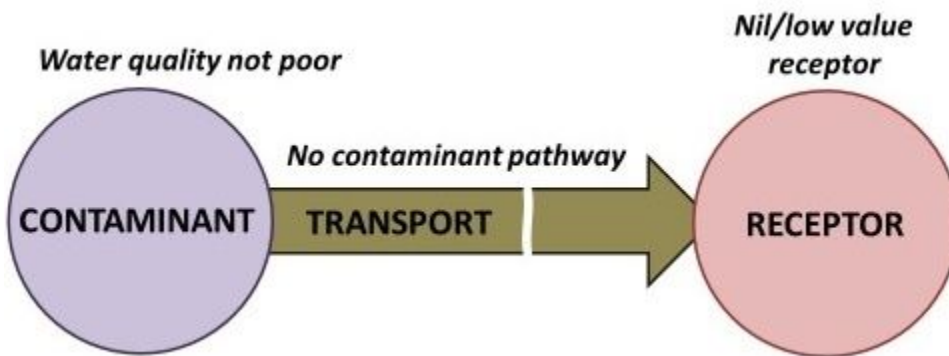
Figure 2.: Contaminant-Transport-Receptor (CTR) model for assessment of pit lake contaminant risk (after DIIS (2016a)).
