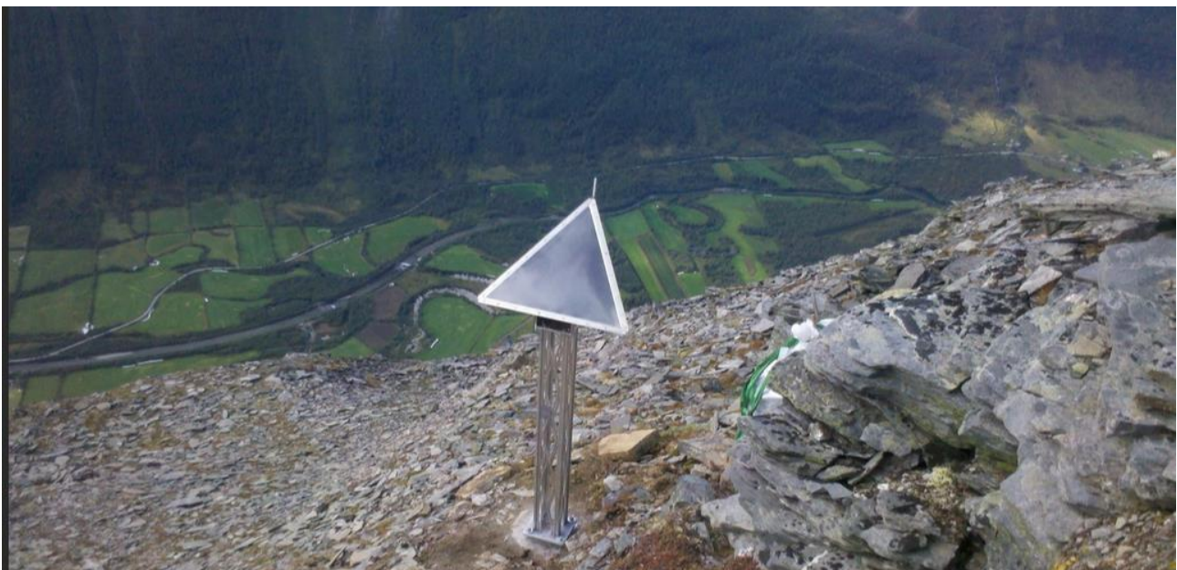
Figure 4 - Example corner reflector (in land based application). Source: University of Bergen, Norway.
