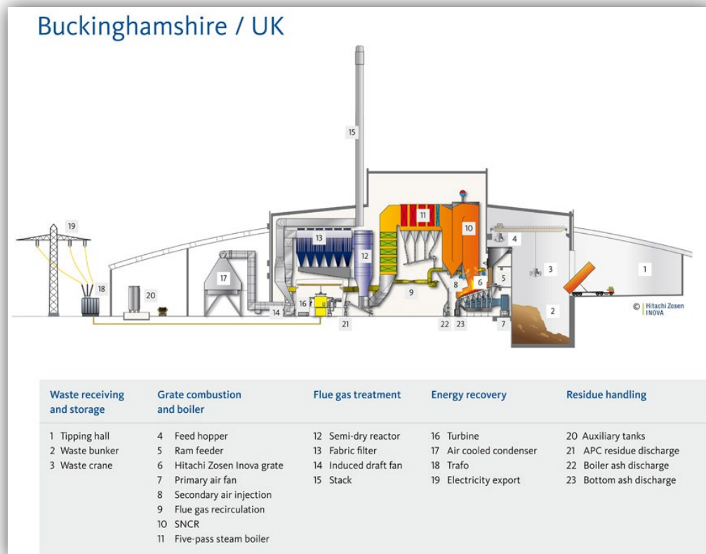
Plate 4 Layout for HZI Buckinghamshire (UK) plant, which is used as a key reference plant for the East Rockingham WtE plant design and planning 1
