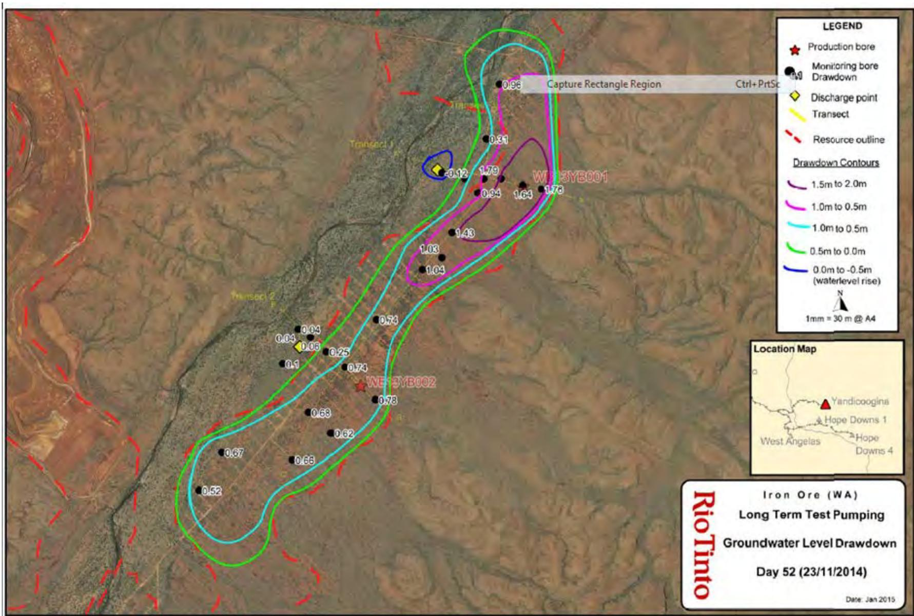
Figure 3-2: Long term Test Pumping groundwater level Drawdown Day 52
