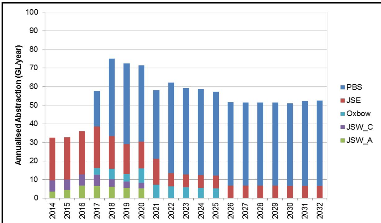
Figure 6-5: Predicted Total Yandicoogina Operations Dewatering requirements (by pit)
