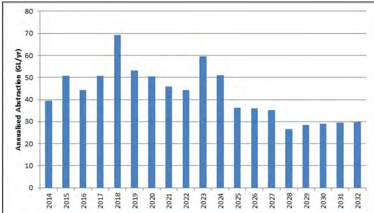
Figure 6-2: Predicted dewatering requirements for the Proposal with no discharge from HD1 flowing in Weeli Wolli Creek
