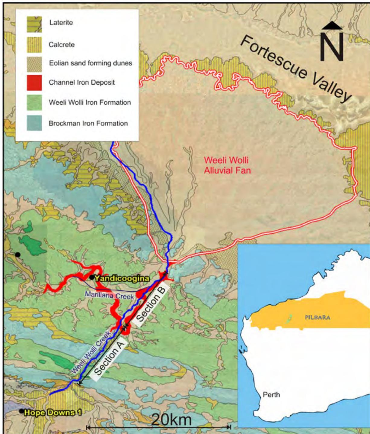
**Figure 2-2: Geological map showing the Weeli Wolli Creek System and the CID Aquifer relative to the Fortescue Marsh**
