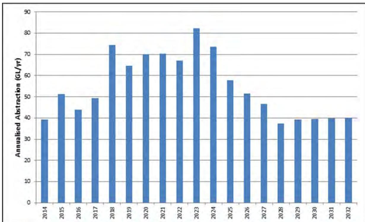
Figure 6-1: Total Yandicoogina Operations Dewatering requirements
