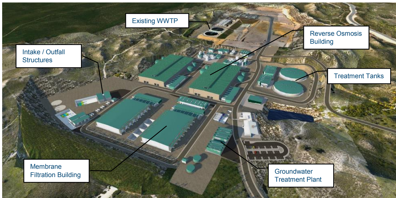
Figure 3-8: Model of ASDP indicative site layout (full plant capacity)
