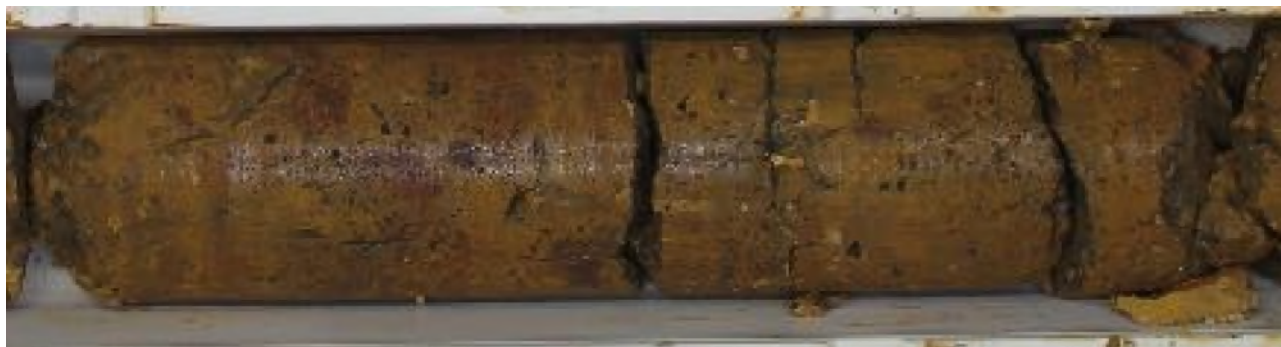
Figure 3.38: Diamond core of CID-upper layer depicting vugs and fractures (CZR 2023)
