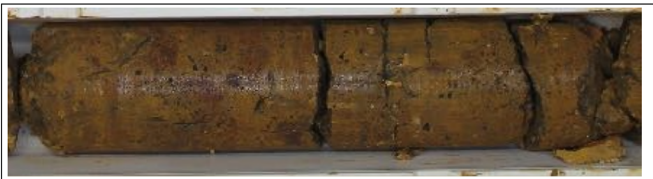
Figure 8.4.26 : Diamond core of CID-upper layer depicting vugs and fractures (CZR 2023)
