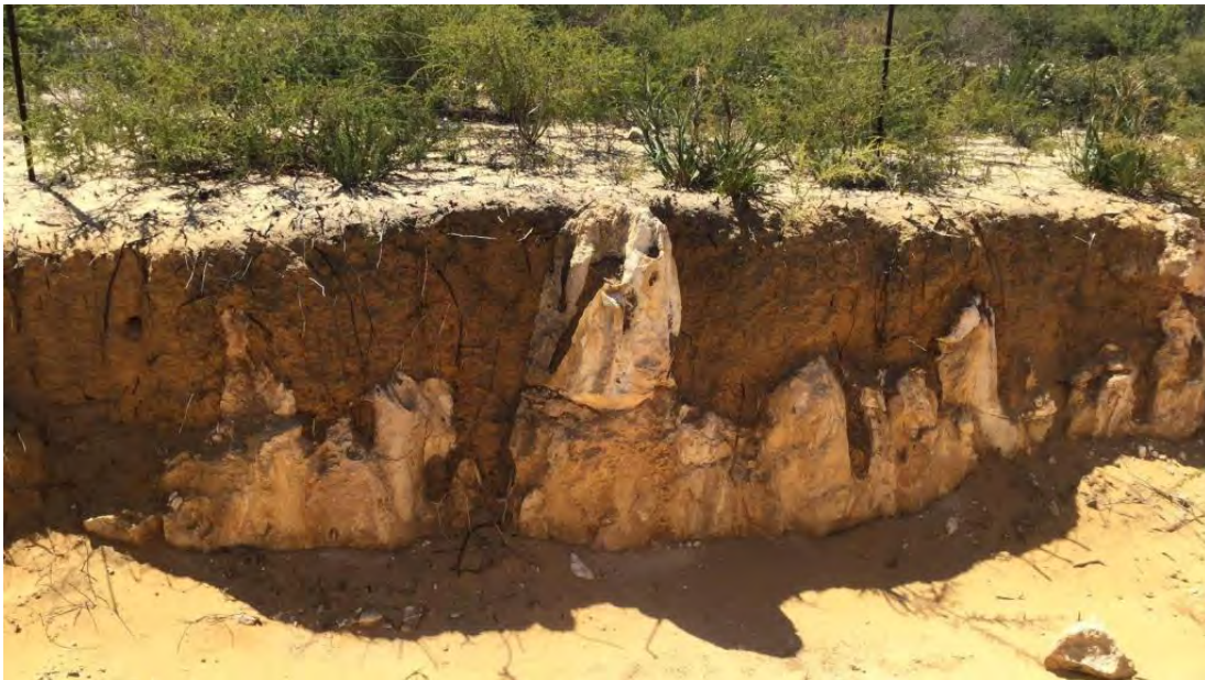
Figure 5-8: Buried pinnacles of Tamala Limestone with sub-vertical solution features ('solution pipes') exposed in excavation and overlain by Tamala Sand
