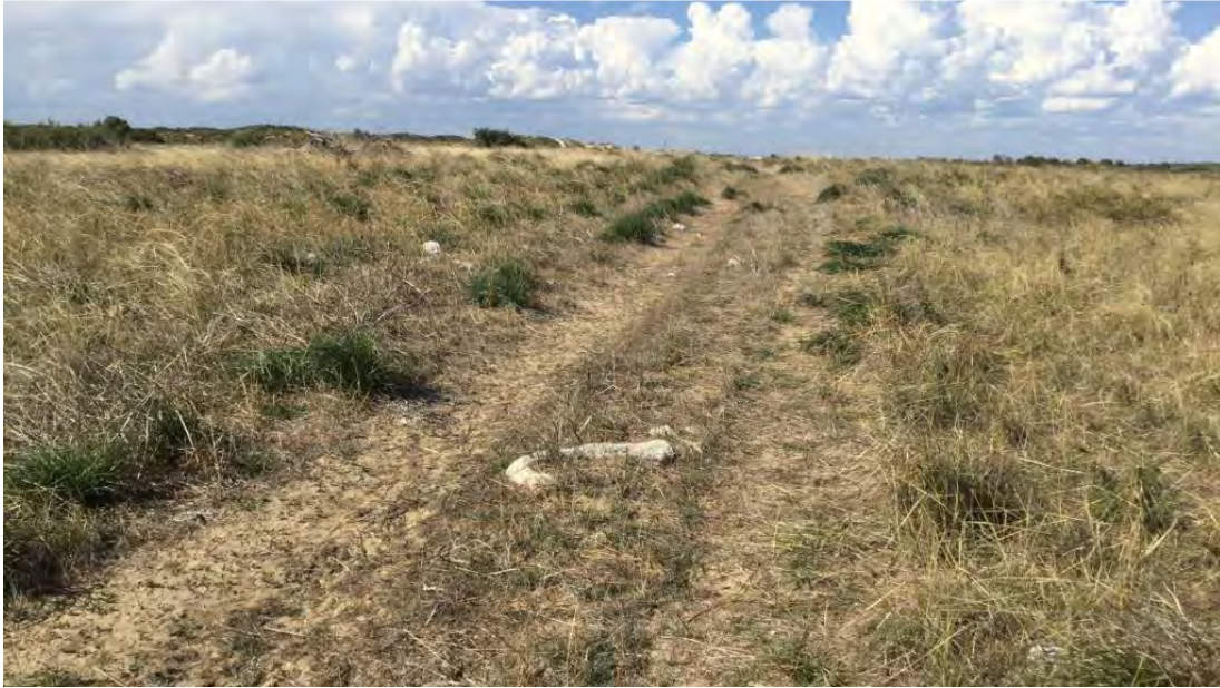
Figure 5-7: Minor surface outcrop of Tamala Limestone indicative of potential buried 'caprock' pinnacles
