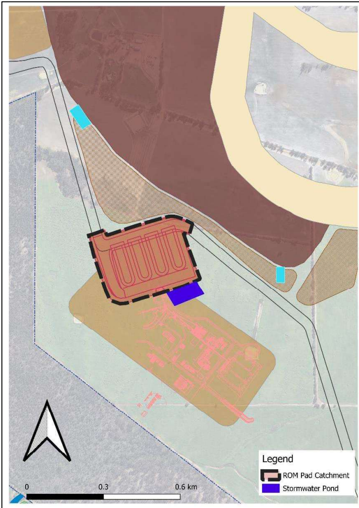
Figure 6.2 Stormwater Pond catchment area and layout
