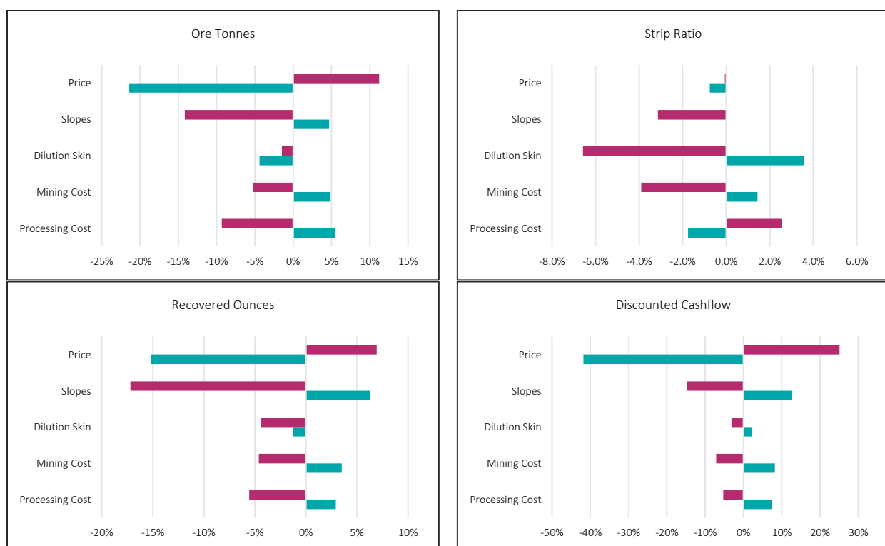
Figure 5-7: Central Zone Pit Optimisation Sensitivity Runs (showing changes with ±10% variance in inputs)
