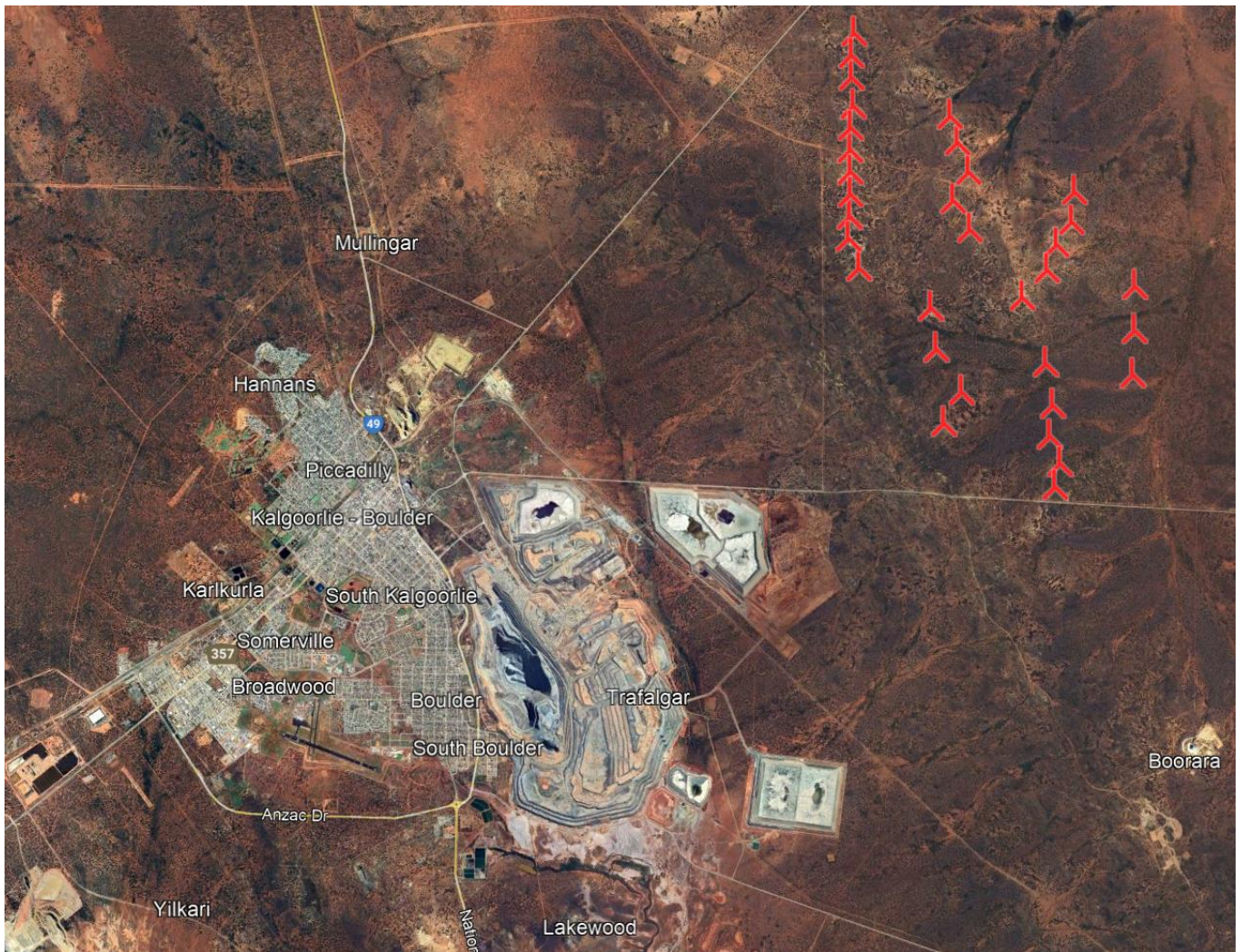
Figure 2 Overview of WTG arrangement for Kalgoorlie Wind Farm: 33 x GW182 7.2/6.2MW – 150 m hub height
