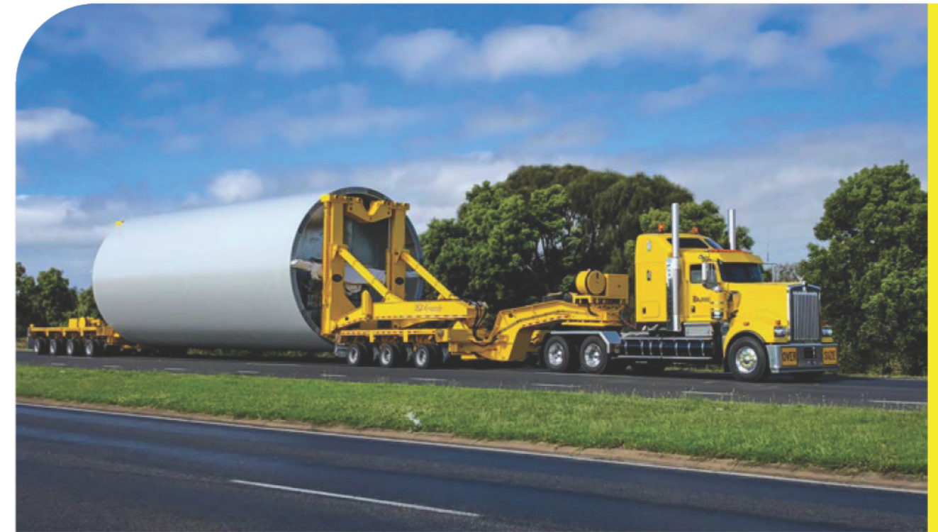
Above: Bookend Trailers used by ARES for Murra Warra's 5.8m towers
