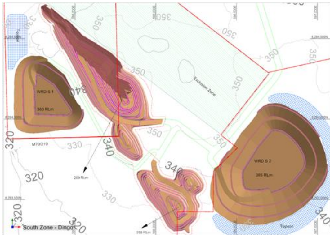
Figure 2-4: Southern Zone WRL Design and Overall Layout
