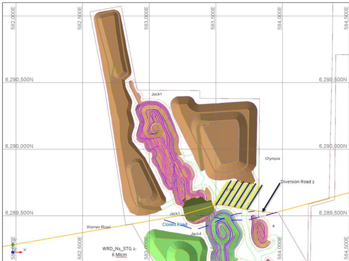
Figure 5-5: Northern Mining Area and Warren Road Solution
