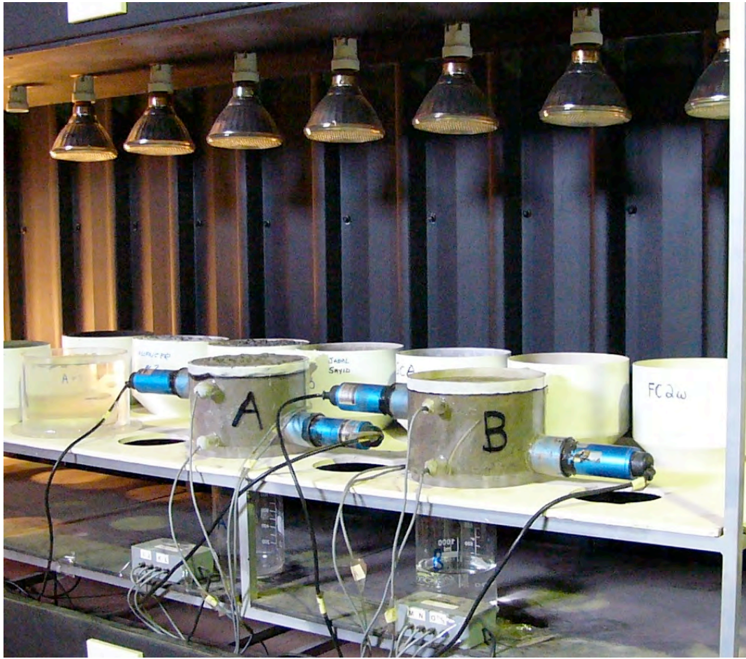
Plate 2: GCA-Research Project: Instrumented-Weathering-Column with -4.75mm Fraction of Trace-Sulphide/Calcareous-Basalt-waste-bedrock Sample.
