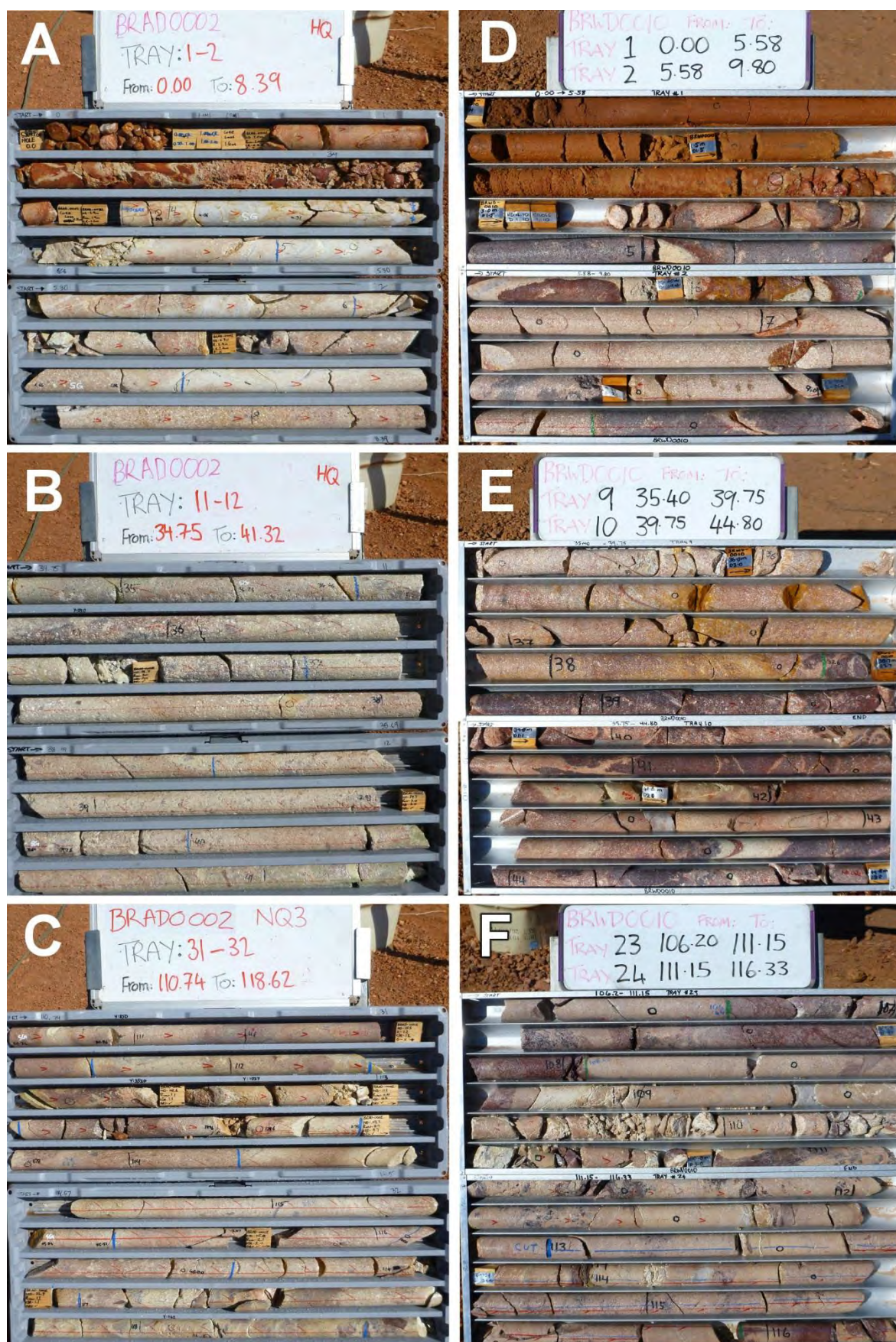
Figure 15: Diamond drill core images within Browns Range Metamorphics; Area 5 drill hole BRAD0002 (close to BRAR0019) — A) 0 to 8.39 mbgl ; B) 34.75 to 41.32 mbgl ; C) 110.74 to 118.62 mbgl; Wolverine drill hole BRWD0010 (close to BRWD0010) — D) 0 to 9.8 mbgl ; E) 35.40 to 44.8 mbgl ; F) 106.2 to 116.33 mbgl.
