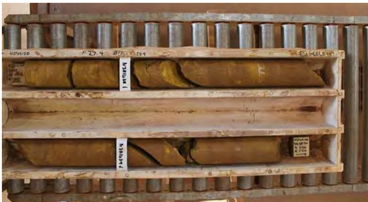
Figure 2. Example of hardcap from the Study Area, demonstrating a lack of vugs. Note that fractures are an artefact of the drilling process.
