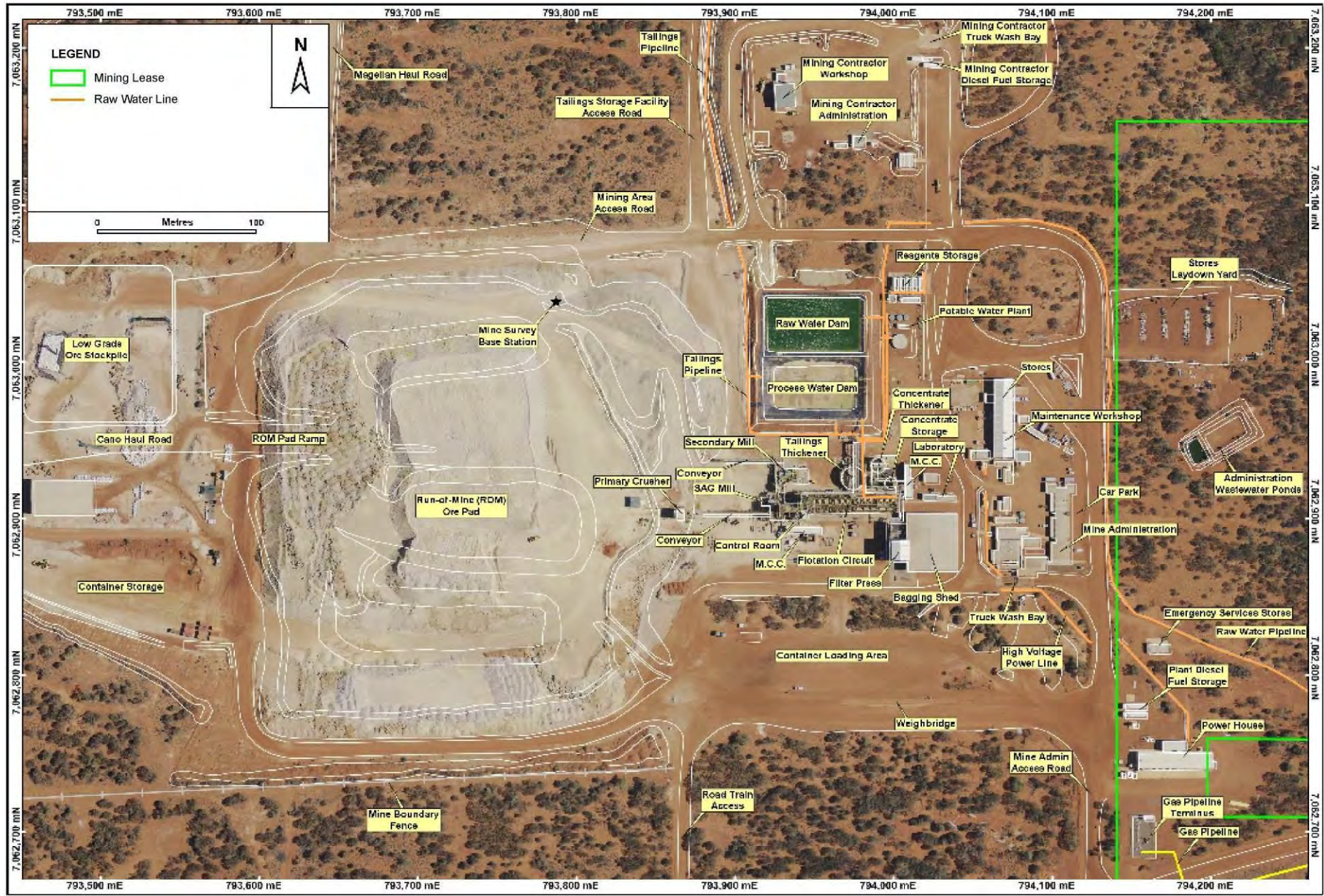
Figure 19 Magellan Lead Carbonate Project plant layout
