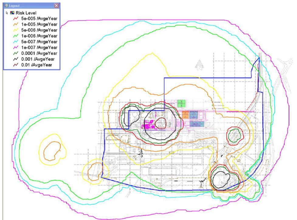
Figure 7 provides the revised site individual fatality risk results (GHD) with the inclusion of the proposed AN #3 facilities, while increasing ammonia imports to 14 per annum.
