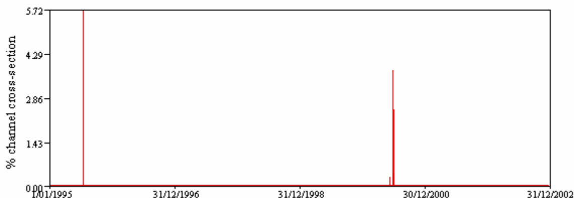
Figure 30. Flow hydrograph showing frequency and magnitude of events when active channel flows occurred (> 0.45 m 3 /sec) during available flow record (1995 – 2002).
