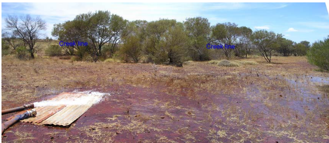
Fig 7. Discharge and spread at the “steep” site (Slope 1.75%). Note creek line (indicated by the row of trees) in background. The water did not flow towards this creek, but sheeted parallel to and away from the creek.
