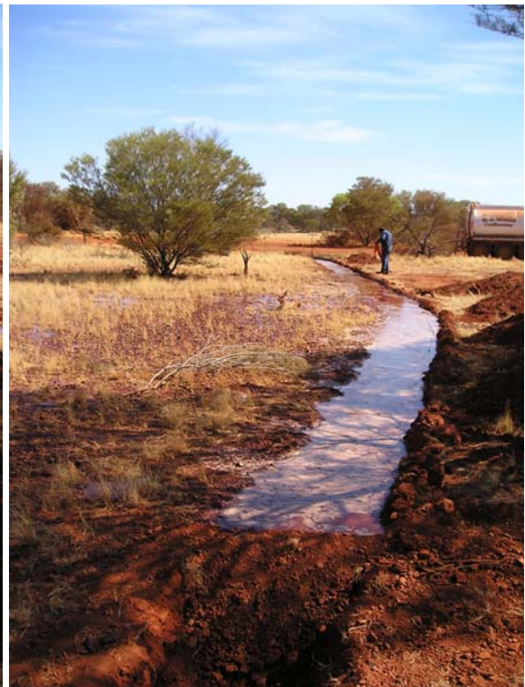
Fig 9b: Reduced flow. Discharge at low point only.
