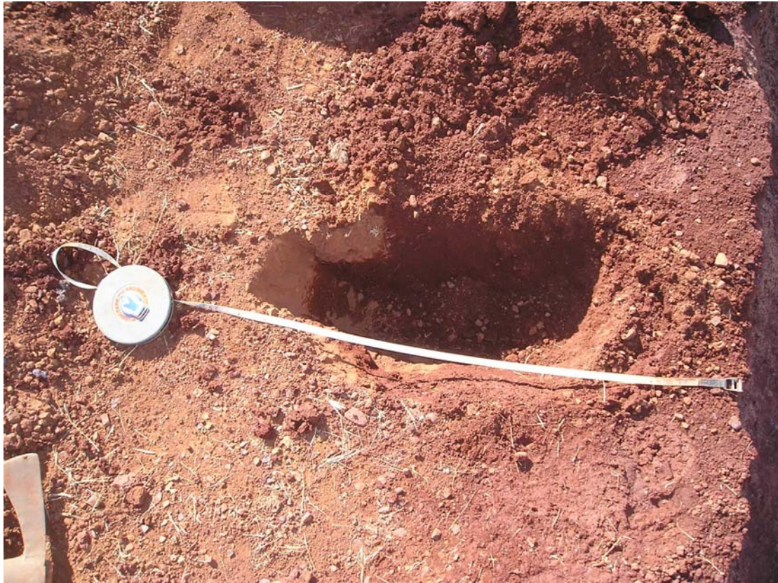
Fig 17: Extent of lateral moisture movement through the soil in 24 hours. Maximum movement was approximately 150mm below the surface. Moisture content 2cm to the left of the obvious boundary was 4.3%.
