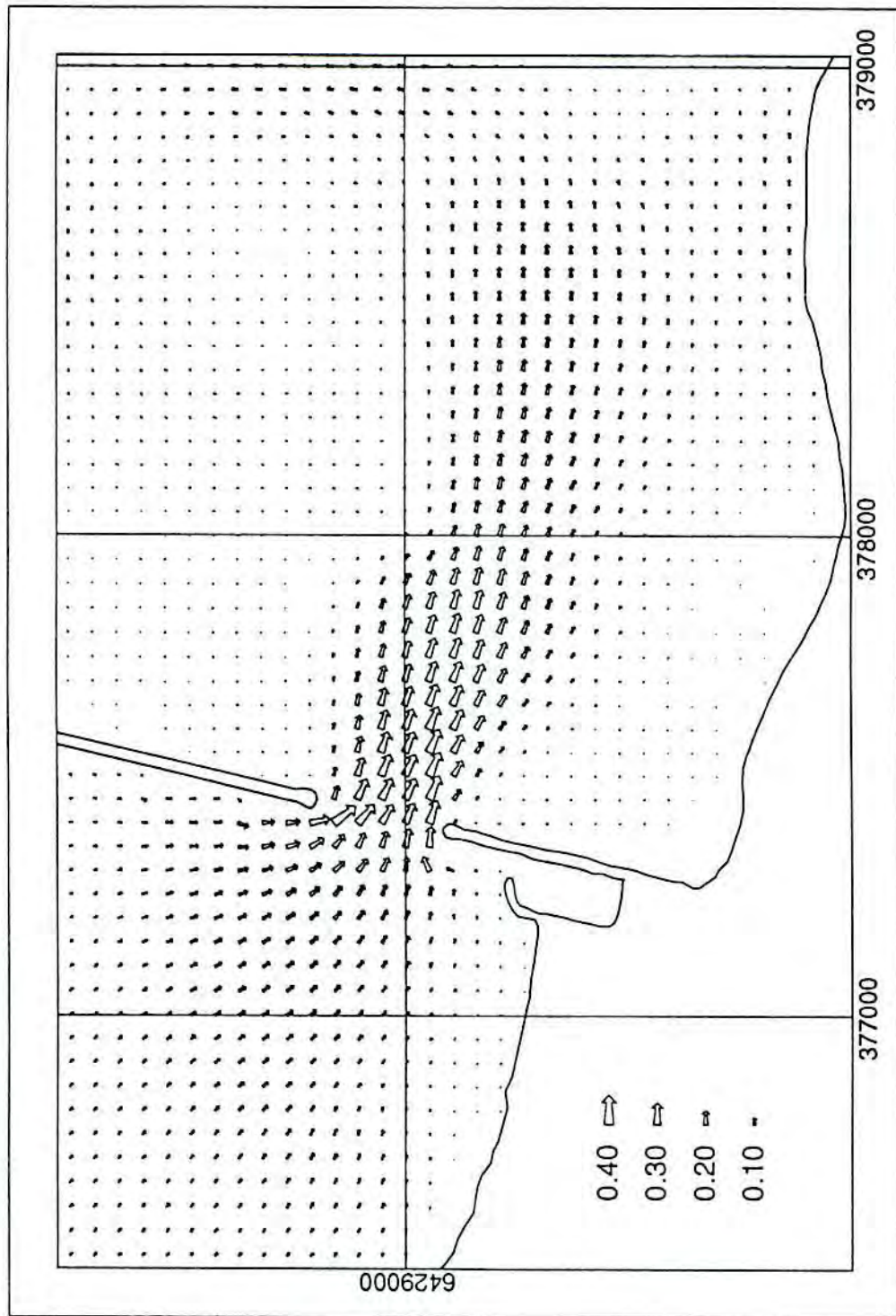
Figure 5 Currents ( \text{ms}^{-1} ). Run 3. Marina absent. Tidal flow : 250 \text{ m}^3\text{s}^{-1} . Wind : 5 \text{ ms}^{-1} from 225^\circ (southwest).
