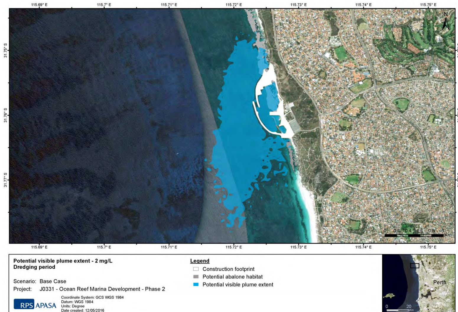
Figure 10.13 Map of the potential extent of the area where visible plumes may occur during the dredging phase at any time (at any particular time, the plume would only cover fraction of this area). Analysis based on TSS elevation of 2 mg/L above background occurring at any time and at any level in the water column.
