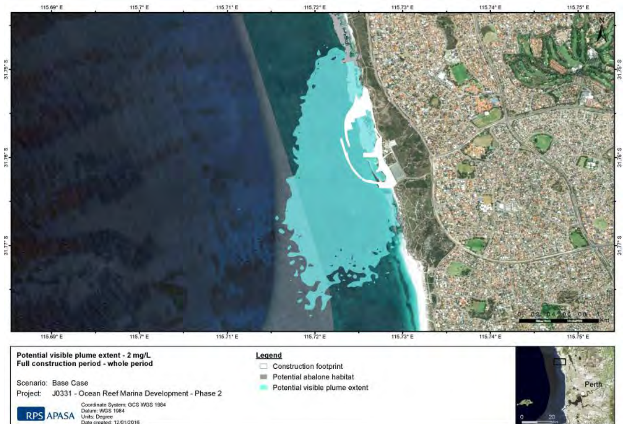
Figure 5.1 Conservative depiction of the Zone of Influence - i.e. potential extent of the area where visible plumes may occur during the full construction period. Analysis based on TSS elevation of 2 mg/L above background occurring during construction at any time (100th percentile) and at any level in the water column. (Source: RPS APASA 2016)
