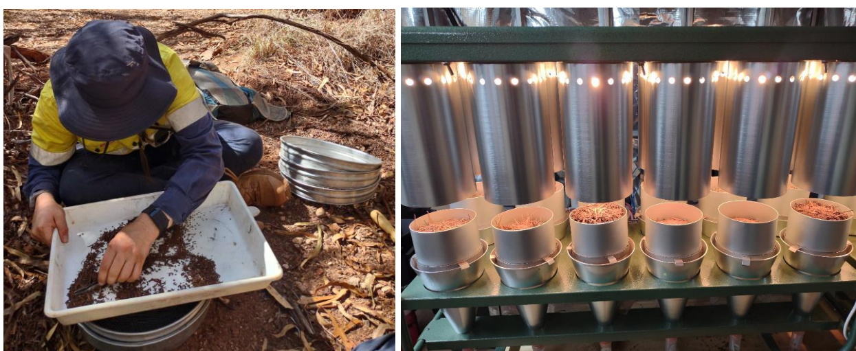
Plate 2.1: Leaf litter and Topsoil Sieving & Tullgren Funnel Set-up
