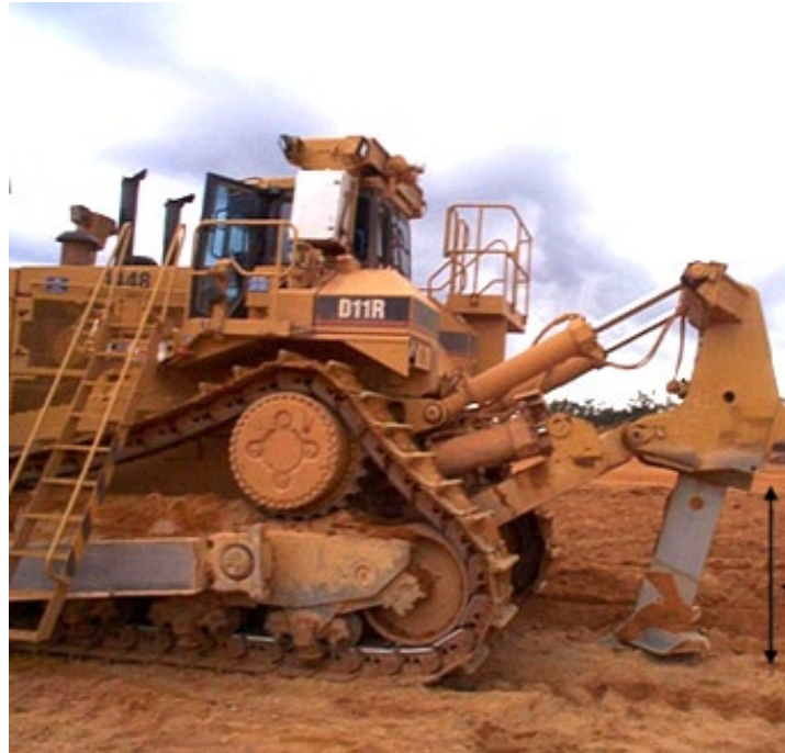
Figure AA-10: Winged tine ripping
