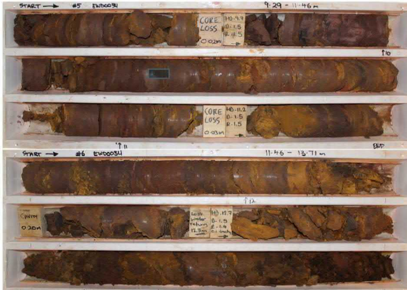
Figure 6.5: Core showing cavities and core loss (potential habitat) at EWD0034.
