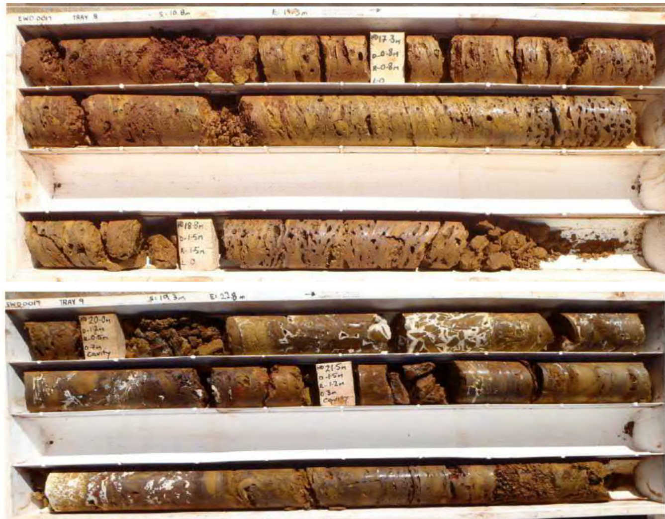
Figure 6.16: Diamond core from hole EWD0017, showing vugs from secondary weathering (highly suitable habitat)
