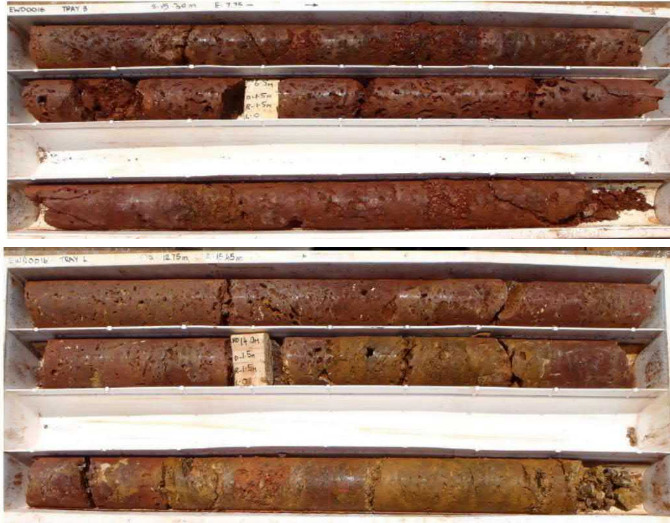
Figure 6.19: Core at EWD0016 showing vugs from secondary weathering (potential habitat)
