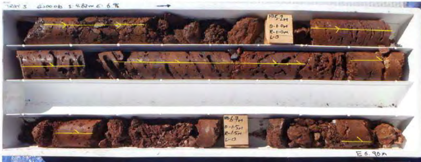
Figure 6.7: EWD0010 Core showing secondary weathering (potential troglofauna habitat) at West End Pit.
