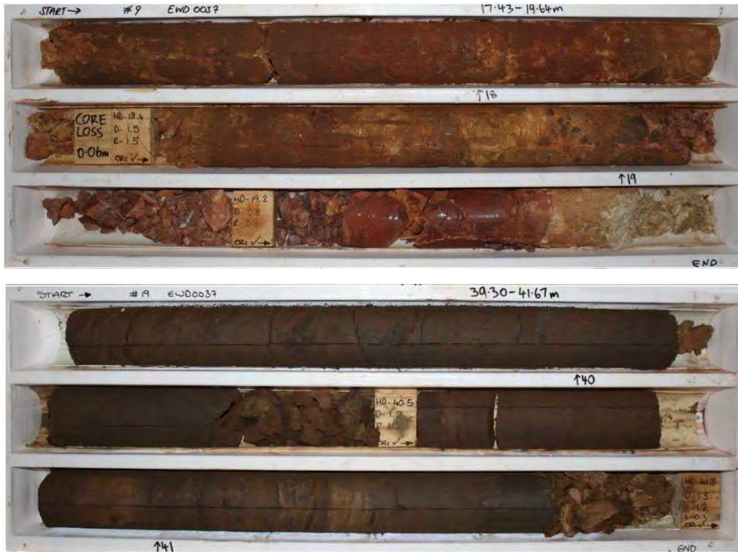
Figure 6.9: EWD0037 Core at Talisman Pit showing core loss in surficial unconsolidated detritals (potential habitat), and fresh shale rock at depth (unsuitable habitat).
