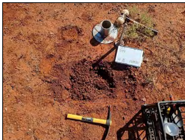
Plate 1: Triaxial surface sample equipment
