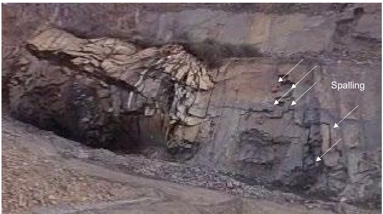
Figure 11 Quarry with 10 m bench height demonstrating spalling adjacent to a blast firing (Slate Quarry)
