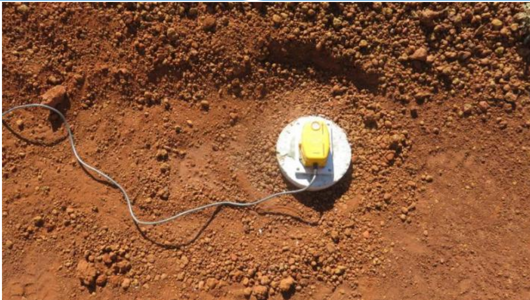
Figure 22 Blast Monitor - Microphone and Geophone Installation
