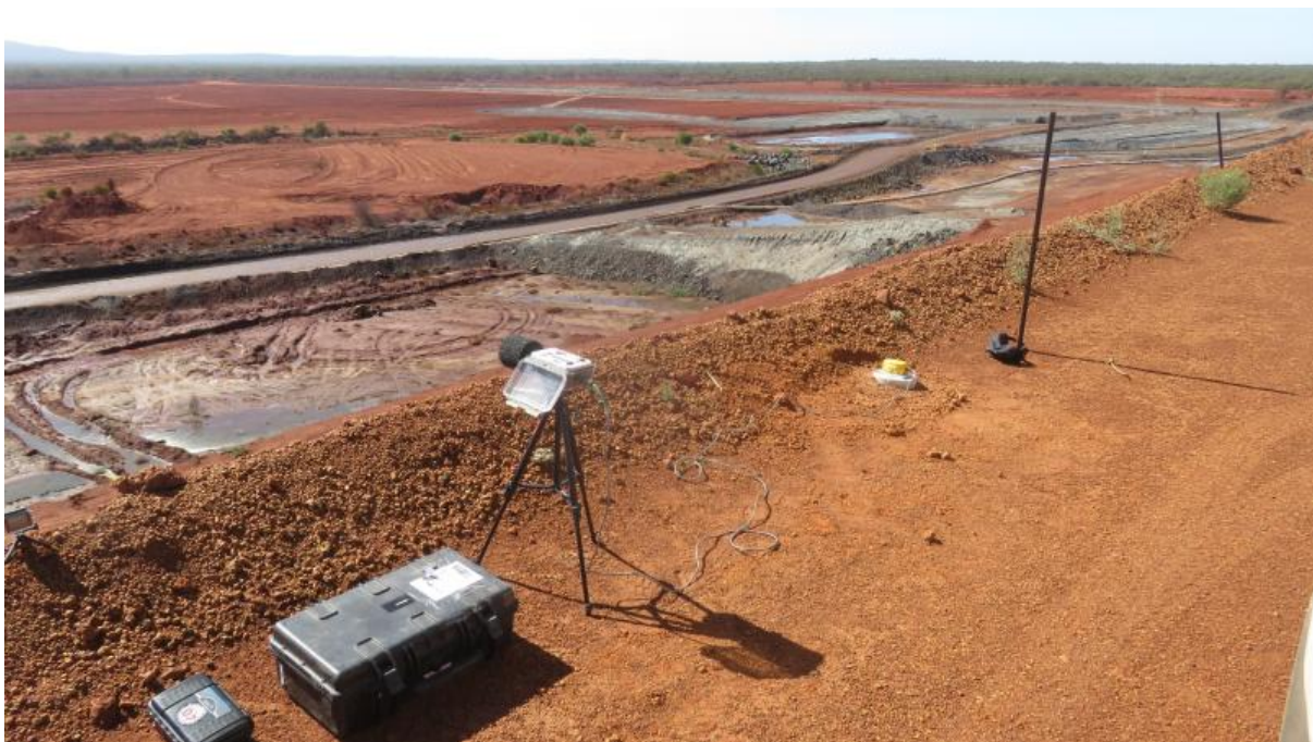
Figure 21 Blast Monitor - Day Use Installation with Permanent Mounting Block
