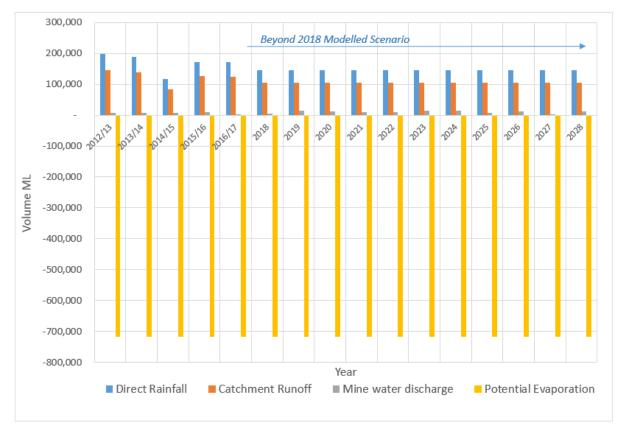
Figure 1: Lake Lefroy key water balance components
