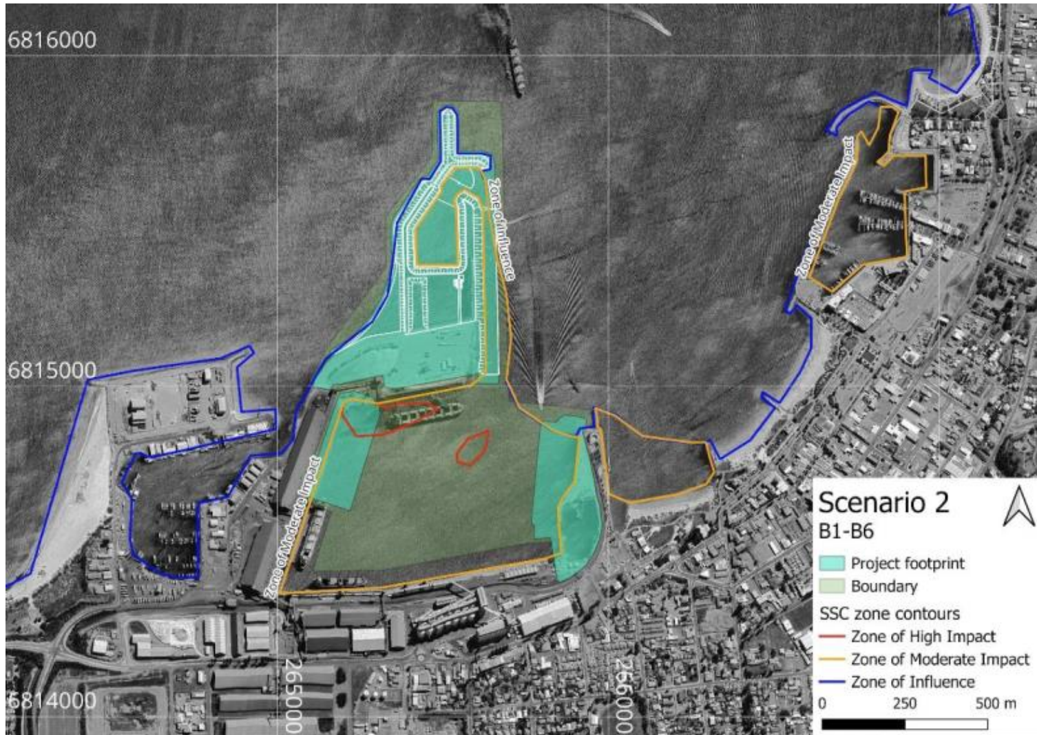
Figure 8-7 Zones of potential impact to BCH during Scenario 2 dredge activities based on SSC criteria proximal to the Port
