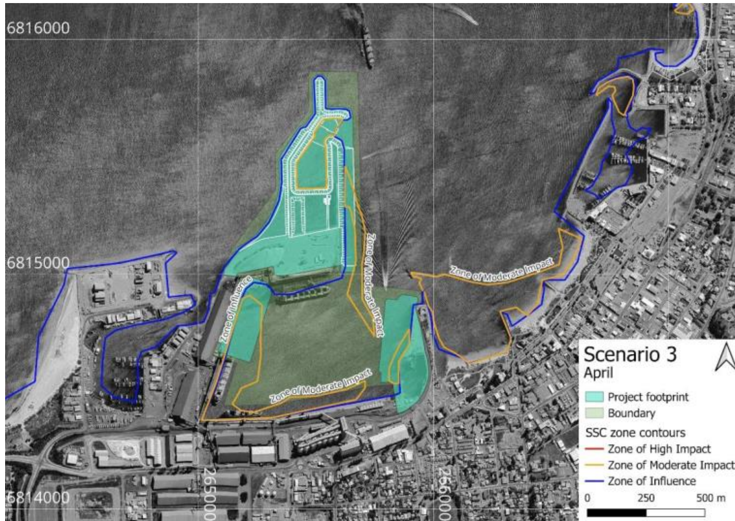
Figure 8-9 Zones of potential impact to BCH during Scenario 3 dredge activities in April based on SSC criteria proximal to the Port
