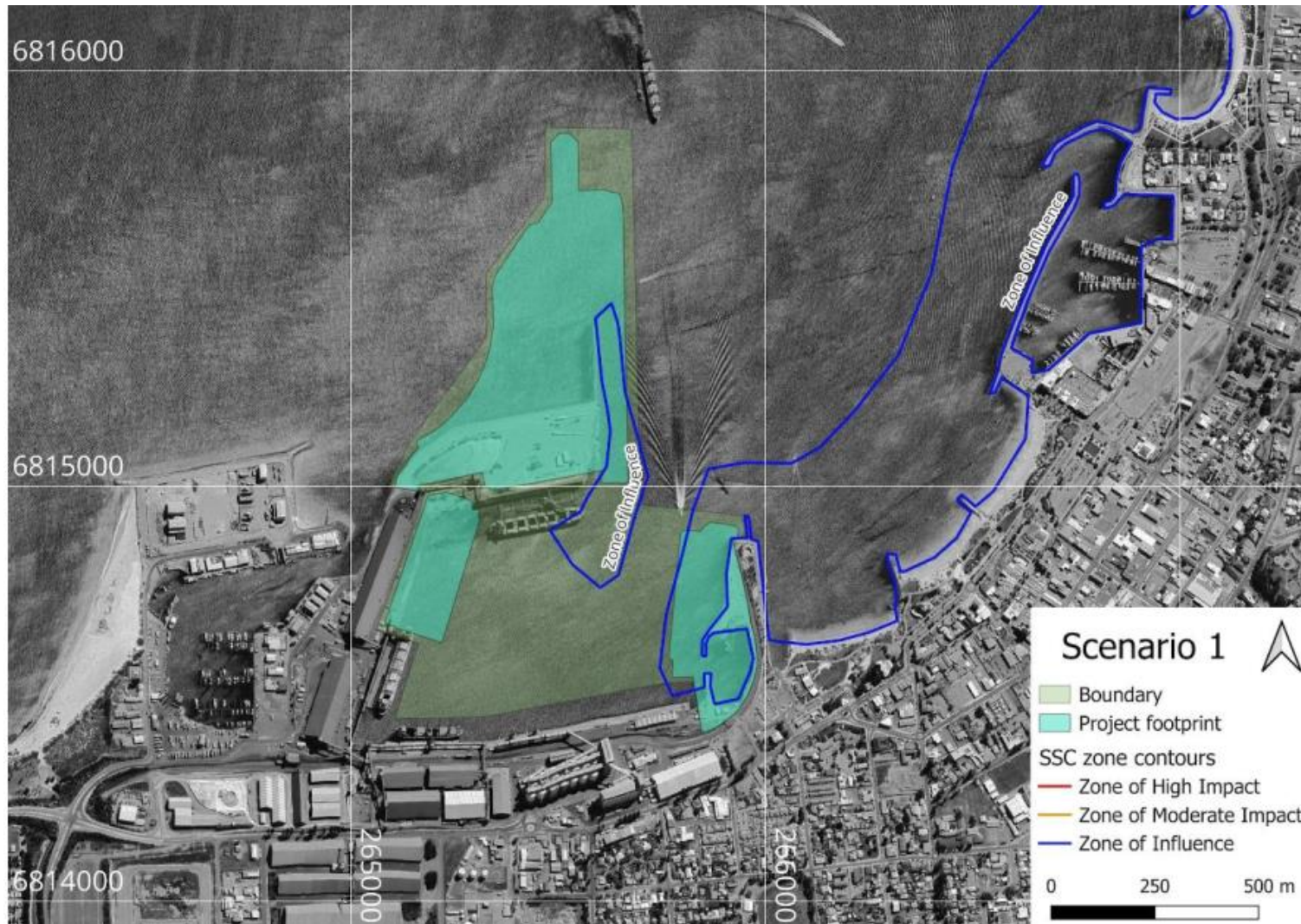
Figure 8-5 Zones of potential impact to BCH during Scenario 1 dredge activities based on SSC criteria proximal to the Port
