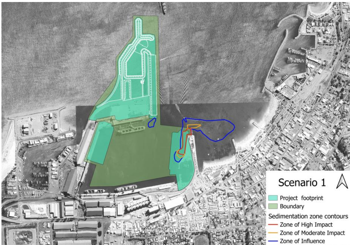
Figure 8-17 Scenario 1 predicted zones of impact associated with dredge derived sedimentation within Champion Bay
