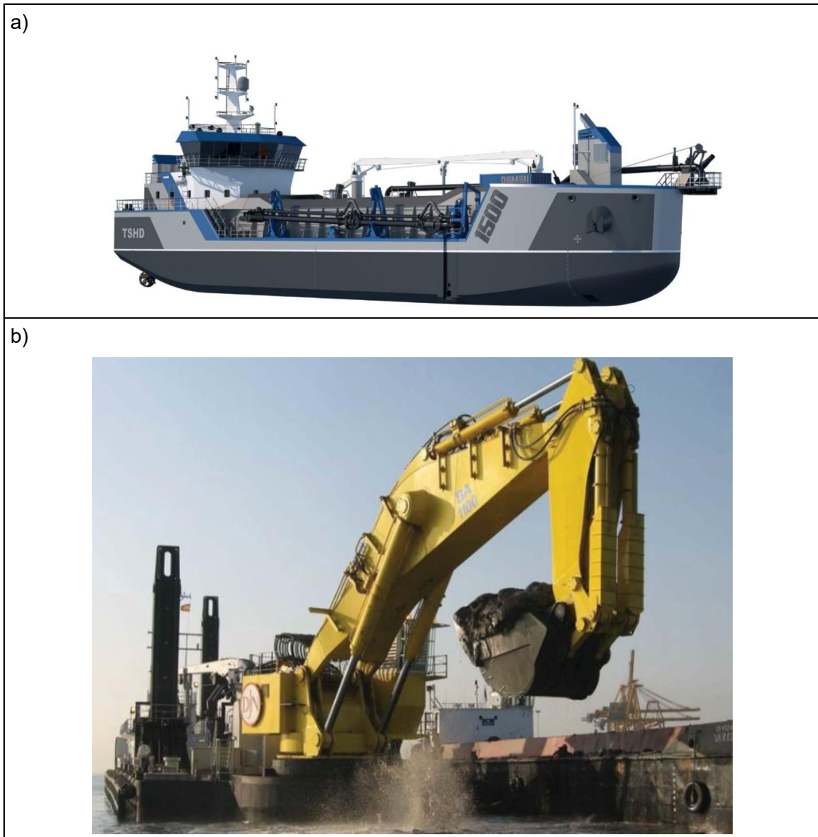
Figure 7-8 Examples of (a) trailing suction hopper dredge and (b) backhoe dredge
